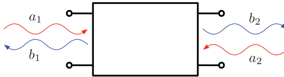
FIGURE A.4 S-matrix relates incoming traveling wave phasors, a_i , to outgoing traveling wave phasors, b_i .
