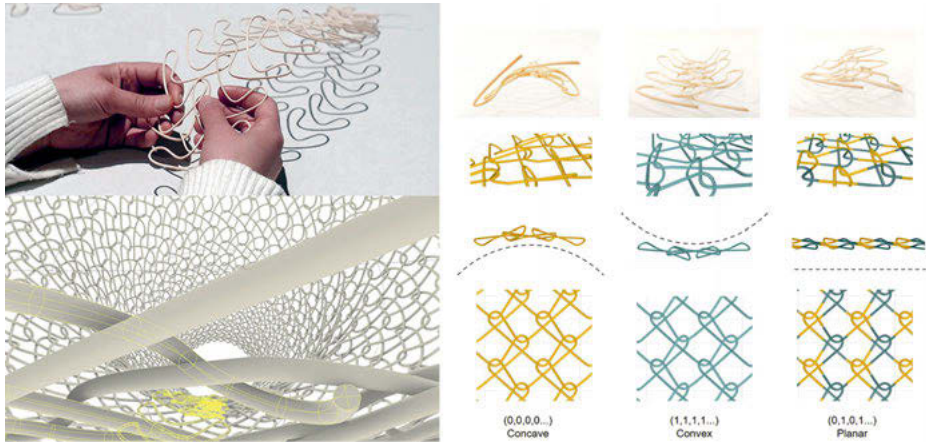
Fig. 4: Structural textile: interlocking order of loops determines the form concave and convex.
