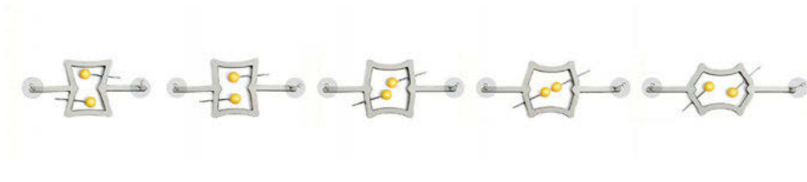
Fig. 3: An inverted hexagonal cell, at increasing stretching, externally fixed to a support (gray circles). The yellow pins showcase the rotation of two opposite inclined walls upon stretching.
