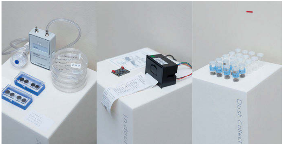
Fig. 5: From left to right: settling dishes, microscopic plates with collections of biotic, abiotic, anthropogenic dust residues for SEM imaging; weekly dust samples collected with cleaning staff at Tieranatomisches Theater (TA T).
