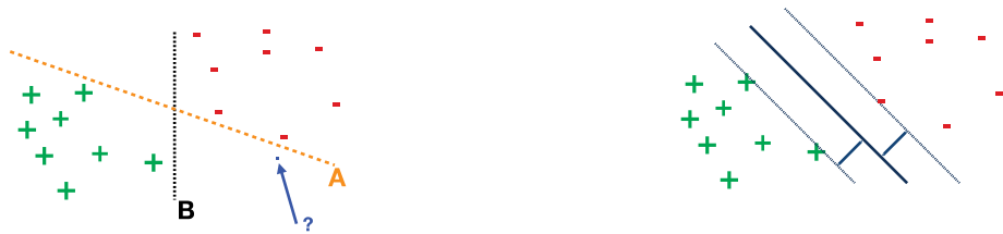
Figure 7.13: Left: two linear separators. Both get unnecessarily close to labeled instances, yielding unintuitive predictions. Right: the max-margin separator keeps the largest possible distance from all instances.
