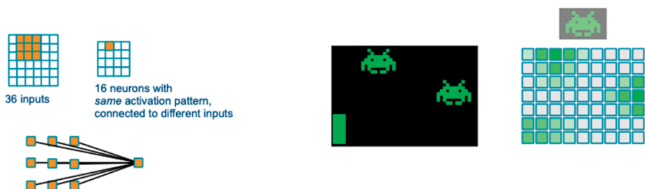
Figure 7.19: A convolutional node is a matrix-valued node that indicates where in the input a certain pattern occurs. Left: a single node in the map is connected to a particular subimage and gets activated when a certain pattern occurs there. Each node in the map has the same activation pattern. Right: illustration of what a map for a particular pattern might look like.
