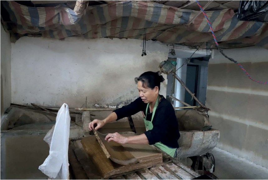
Fig. 13: Pulling the bamboo screen off the wet paper sheet
