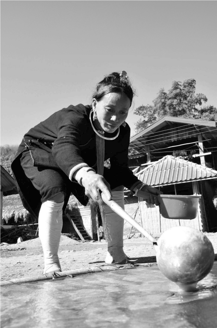
Fig. 9: Solution poured over cotton boards; left to dry for three to four hours (or all day); photograph 2011, Luang Namtha.
