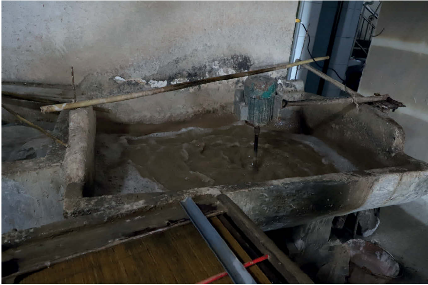
Fig. 9: Fibre pulp being stirred in the trough
