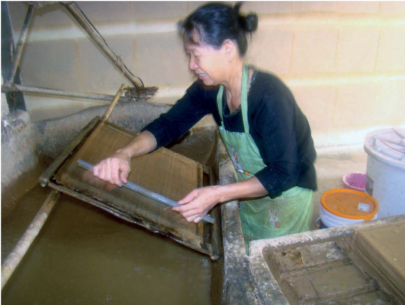
Fig. 12: Trimming the edges of the wet paper
