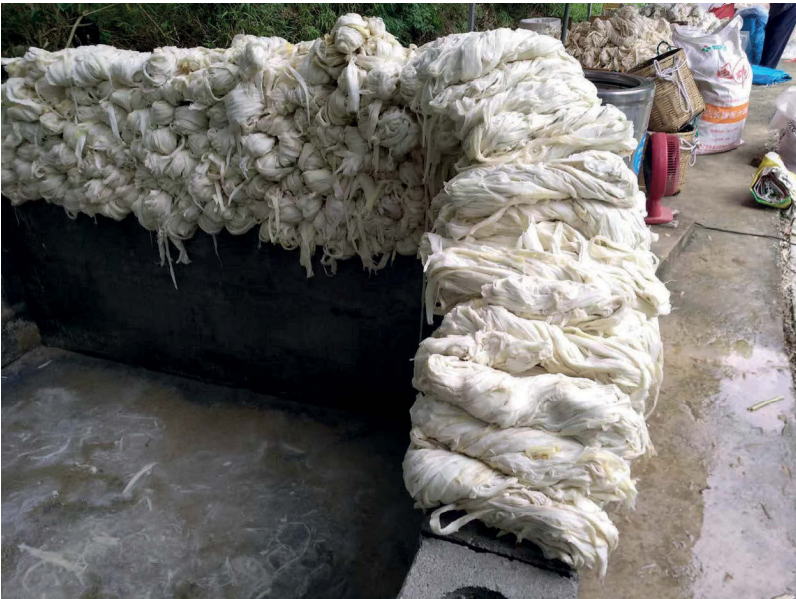
Fig. 8: The processed yarn after rinsing off the lye solution
