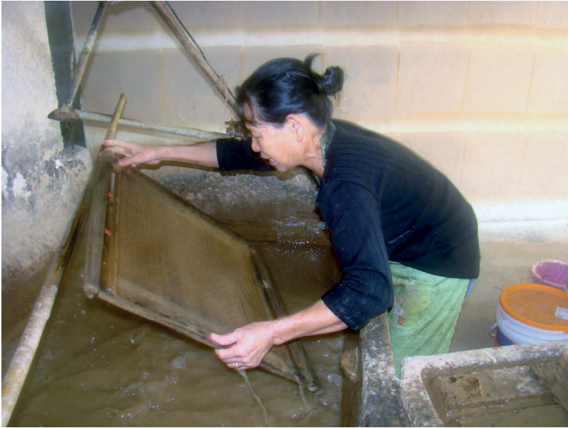
Fig. 11: Taking the bamboo screen out of the water
