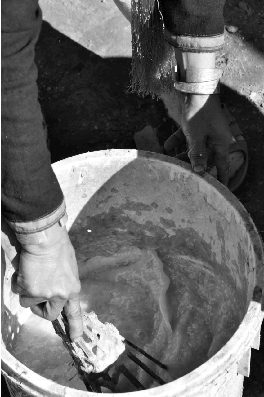
Fig. 8: Pulp mixed with a stick or by hand to suspend the particles of bamboo in the water, and again with a gluing agent made from a native tree; photograph 2011, Luang Namtha.
