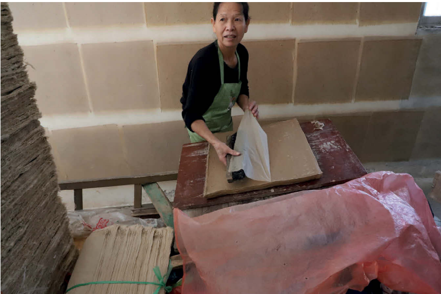
Fig. 14: Peeling off the half-dried paper sheets
