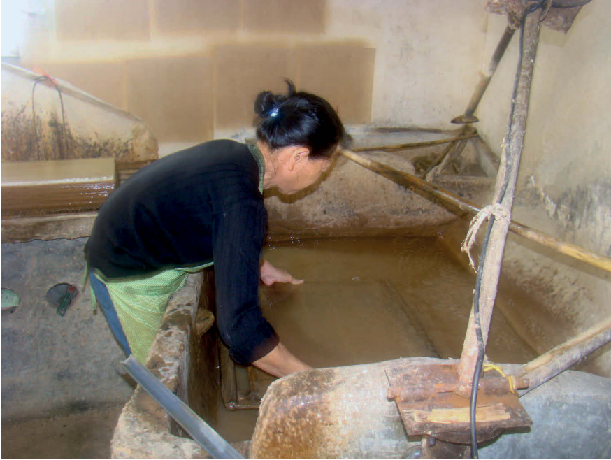
Fig. 10: Scooping up the fibre pulp onto the bamboo screen
