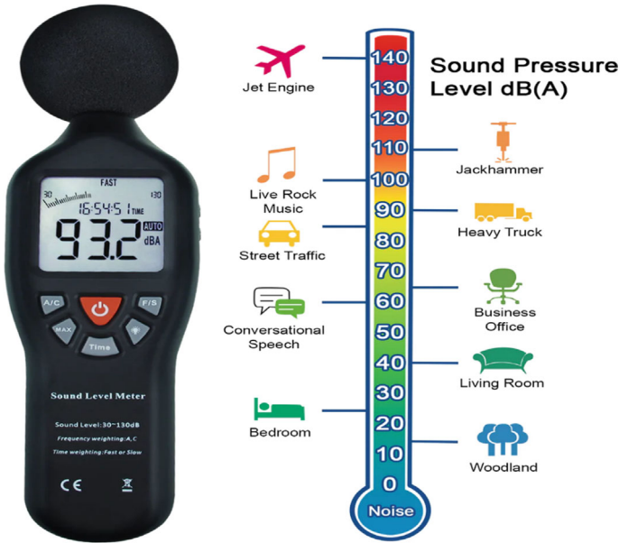
Fig. 2.2 A Sound-Level Meter and examples of decibel levels from different sound sources
