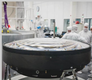
World's largest optical lens (5.1 ft.) built for the 3.2 gigapixel camera of the Vera C. Rubin Observatory, first light expected in 2025 ( https://gallery.lsst.org ), CC BY 4.0
