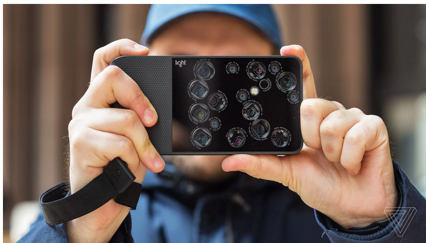
Fig. 2.21 Light L16 camera with 16 camera modules
