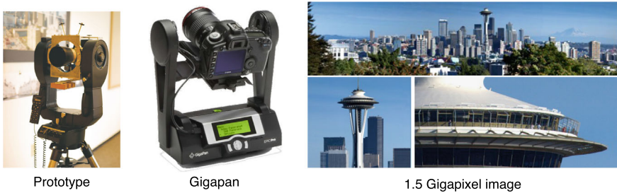
Fig. 3.1 Motor-controlled camera mount for capturing gigapixel images. From left to right, the prototype, the commercial product Gigapan, and the captured gigapixel images of the skyline of Seattle, WA, USA. Reprinted from Kopf (2007)
