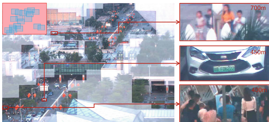
Fig. 2.31 Gigapixel-level videography captured using our UnstructuredCam. The red and blue rectangles on the top left represent the poses of the global and local cameras. The zoomed-in details of three regions at 400, 450, and 700m are shown in the right column
