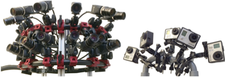
Fig. 2.25 The two unstructured camera arrays used in [21]. Left: 14 Lumenera LT425 machine vision cameras, each recording at a resolution of 2048 \times 2048 . Right: 5 GoPro Hero3 cameras, each recording at a resolution of 1920 \times 1080
