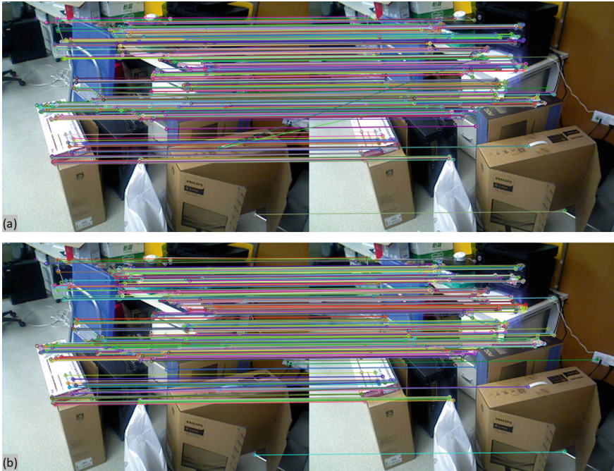
Fig. 5.56 Sparse matching. a Correspondences generated by a sparse matcher [49]. b Correspondences after outlier filtering
