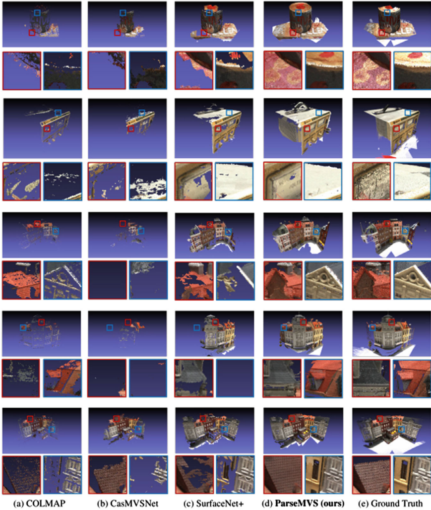
Fig. 5.21 Qualitative comparison for sparsity = 10 , i.e., for an order of magnitude fewer images. We choose 5 scenes from the DTU dataset [1] for visualization
