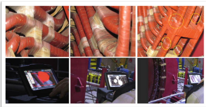
Fig. 11. Analysis of images/spectrum – some evidence (whitened/indicated) detected through UV equipment
