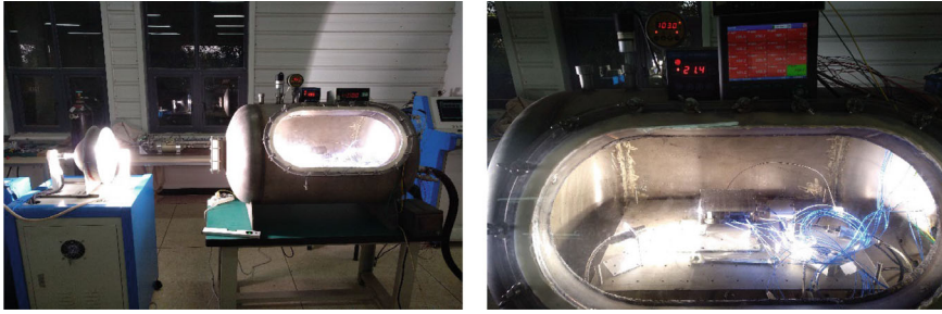
Fig. 9.12 Xenon lamp heating experiment and inside condition
