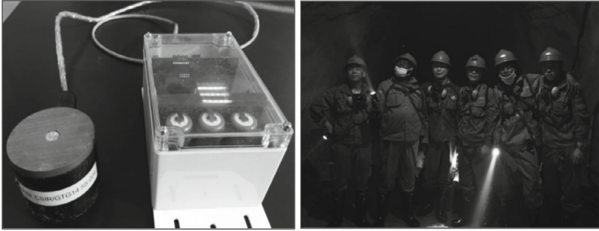
Fig. 8.27 Localized real-time microseismic monitoring equipment and its appliance in Sanshandao Gold Mine
