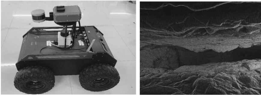
Fig. 8.2 The vehicle-based BLSS 3D laser scanning system (left) and the 3D point cloud of underground mine (right)
