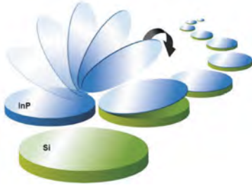
Fig. 3. InPoSi wafer fabrication principle (SOITEC SMARCUT™ process).
