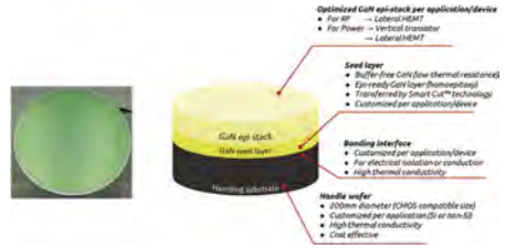
Fig. 12. The SmartGaN substrate stack-up for optimized power or RF applications.
