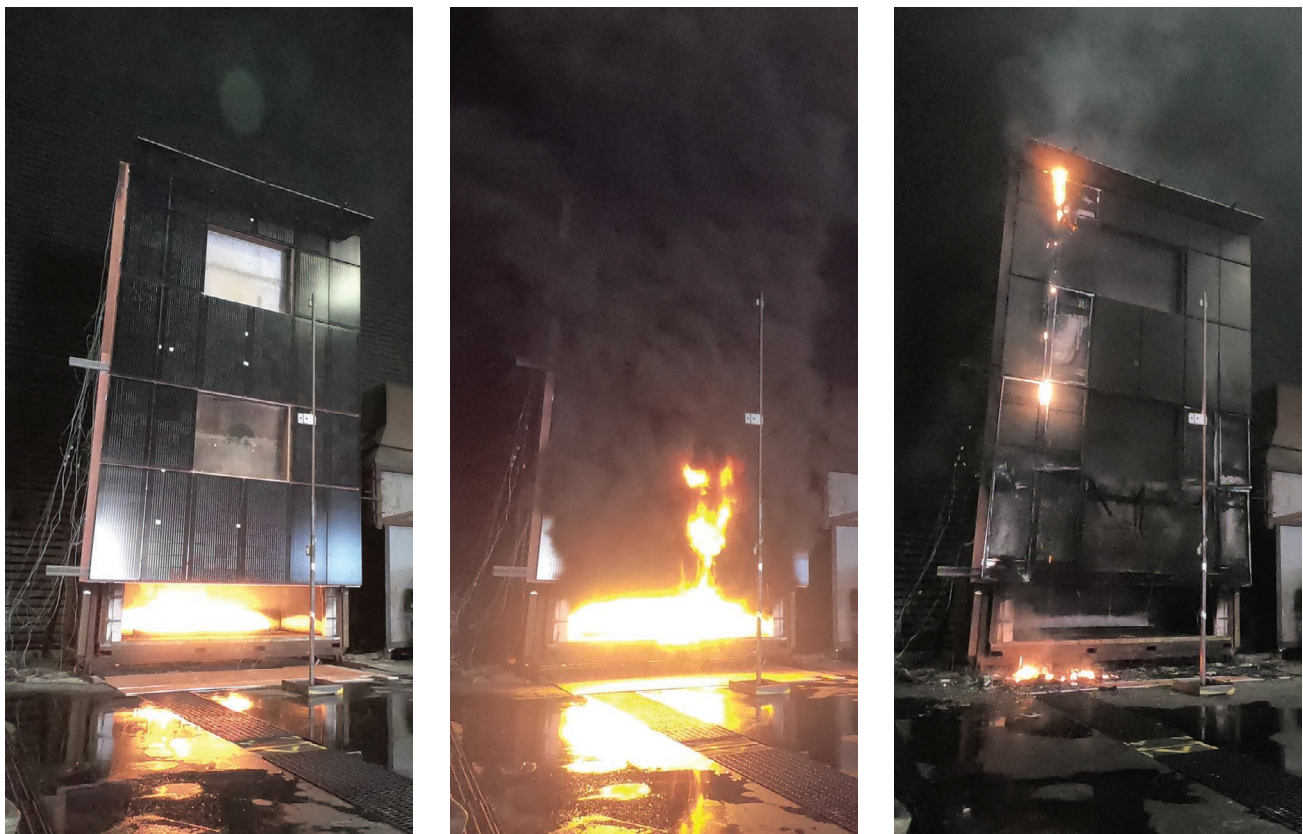
Figure 2.6 Three stages during a large-scale fire test of a BIPV façade according to SP FIRE 105. Photo credits: RISE Fire Research.
