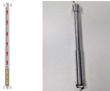
Fig. 2. Distribution load and image of the tendon.
