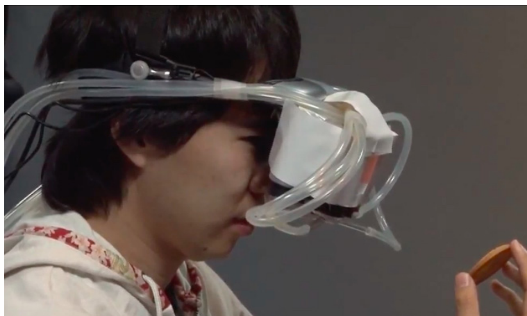
Figure 2: MetaCookie+ allows a multimodal addressing of the visual, olfactory and gustatory sense as well as a bodily-proprioceptive contact with the cookie (cf. MetaCookie at Exploratorium After Dark; https://www.youtube.com/watch?v=Oe39HQH78x4 ).
