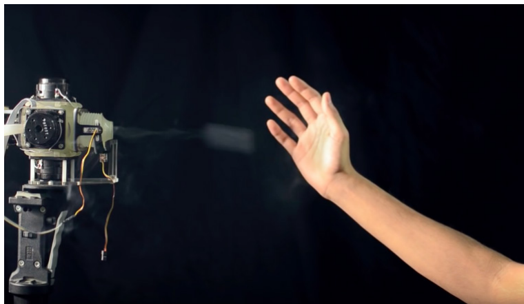
Figure 7: AIREAL of Disney Research uses compressed air for a tactile feedback (cf. AIREAL: Interactive Tactile Experiences in Free Air; https://www.youtube.com/watch?v=xaFBjUJjooM ).
