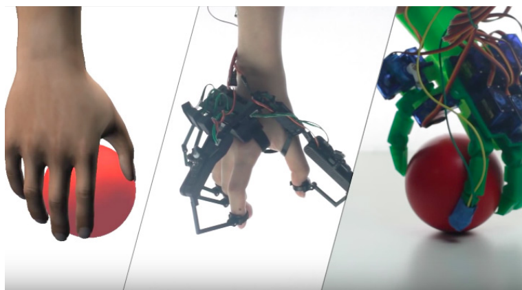
Figure 5: With the exoskeleton of Dexmo Robotics it is possible to grasp virtual objects (cf. Dexmo: an exoskeleton for you to touch the digital world; https://www.youtube.com/watch?v=TPW5OKoc7dQ ).
