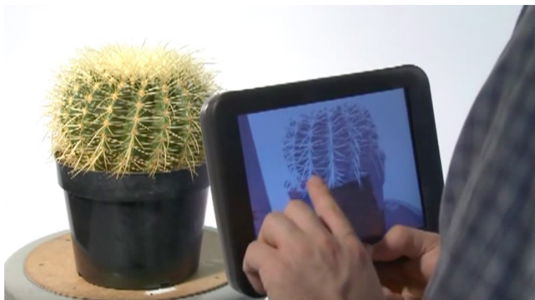
Figure 6: The 3D-Tactile Rendering of Disney Research Pittsburgh uses a display with electro vibration to enable a stimulus-driven force feedback (cf. Tactile Rendering of 3D Features on Touch Surfaces; https://www.youtube.com/watch?v=z01n5CyCKro ).
