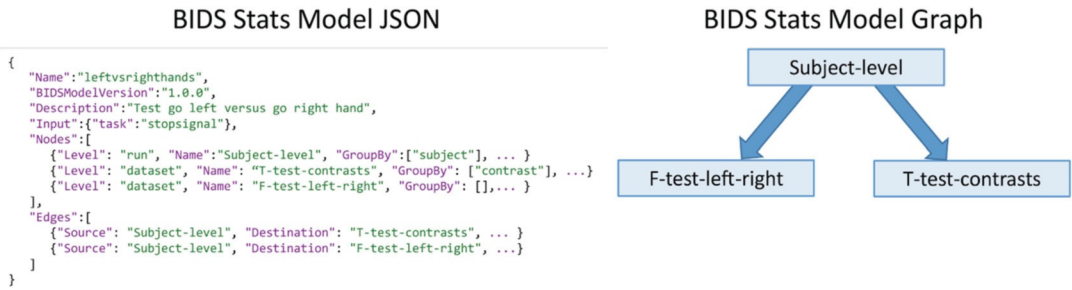
Fig. 4 An example of a BIDS Stats Model for comparing responses between left and right hands. On the left: the JSON model file used as input for FitLins . On the right: the execution graph for the computational model
