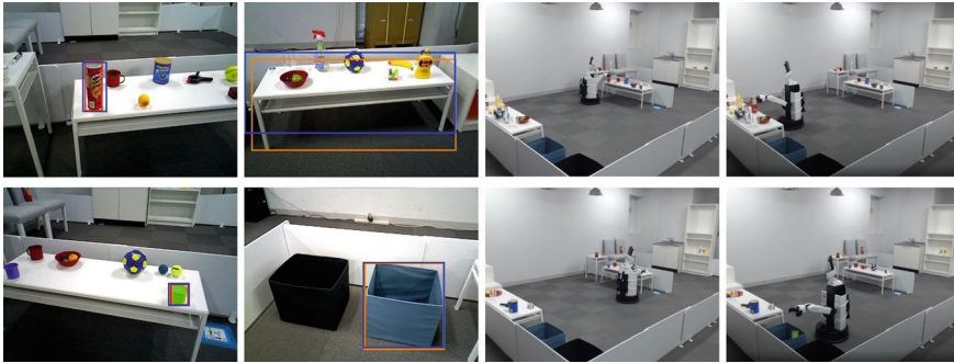
Fig. 5.21 Qualitative results of the physical experiments. From left to right: target object candidate, destination candidate, scene of object grasping, and scene of object placing. Red, orange, and blue bounding boxes represent the ground truth region of the target object, the ground truth region of the destination, and the target object or destination candidates, respectively
