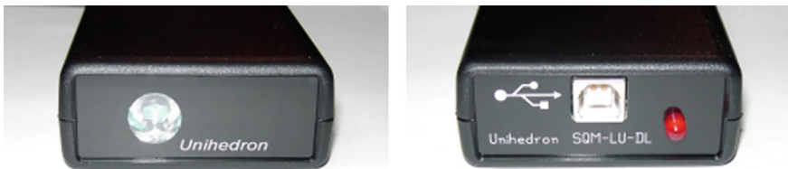
Fig. 2 Sky quality meters with lenses (SQM-LU-DL). Sensors to quantify the lunar irradiance and light pollution
