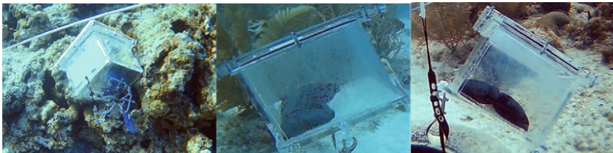
Fig. 4 Installation of the lunar light sensor to 11 m depth in a Johnny Cay, b Acuario, and c West view. Photos: Andrés Felipe Chilma
