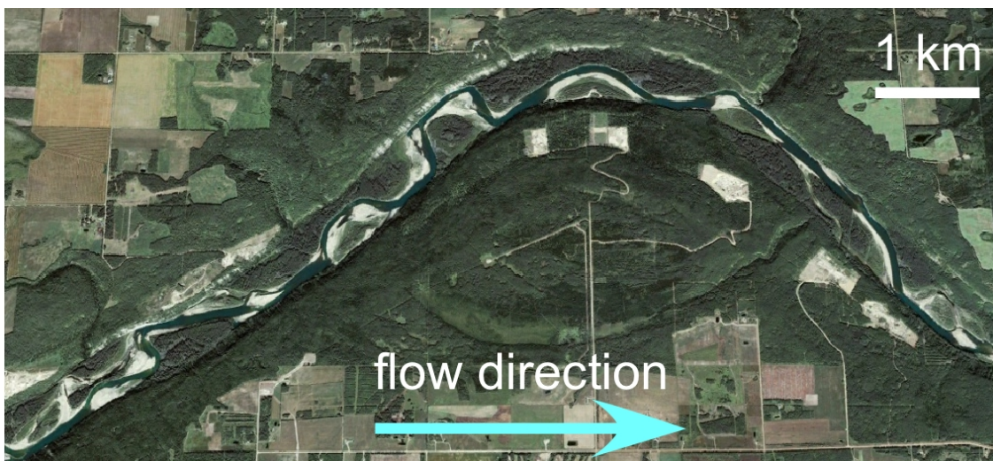
Figura 11. The equilibrium meander train formed in the Beaver river (Canada) whose planform evolution is constrained by the valley walls. (Credit: Google Earth. lat. 54^{\circ} 22' 49.6'' N; lon. 110^{\circ} 15' 36.9'' W).
