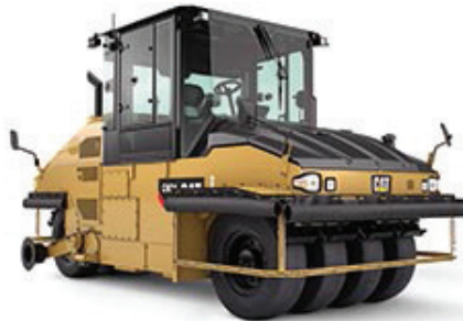
Figure 8-3. A typical pneumatic tire roller. Tire pressure can be adjusted by the operator to optimally compact the lift of the material.
