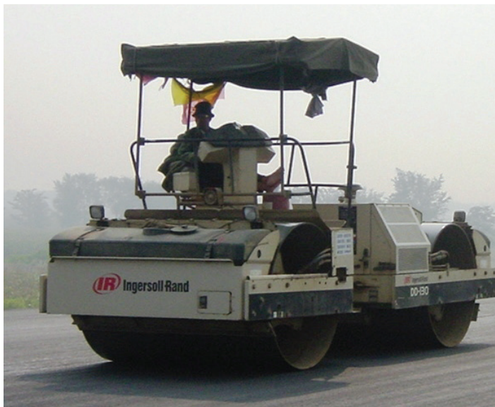
Figure 6-22. Smooth-wheel roller. This roller compacts fine-grained soils and finishes the surface of asphalt pavement.
