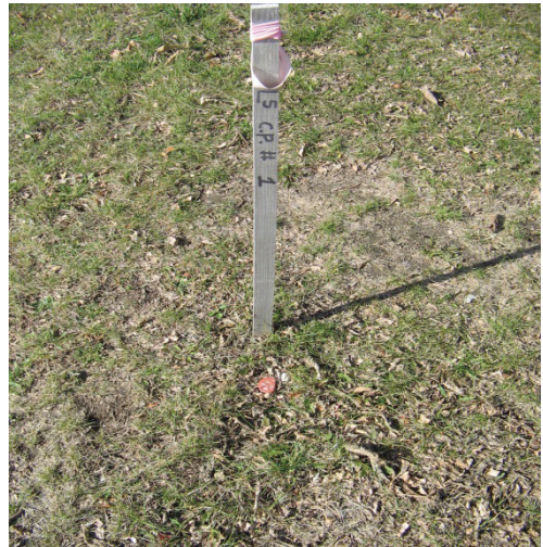
Figure 5-4. Contractor primary control.
