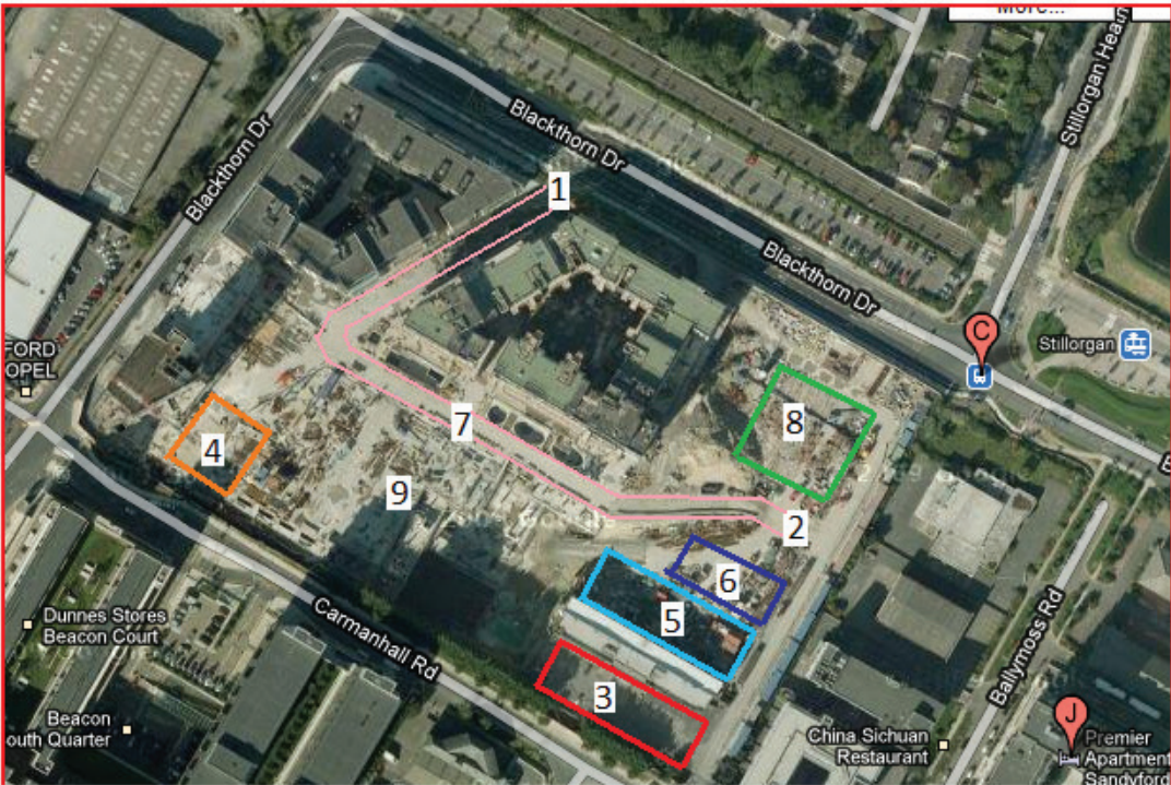
Figure 4-36. The final site organization and layout for the site drawn over the Google Earth image.
