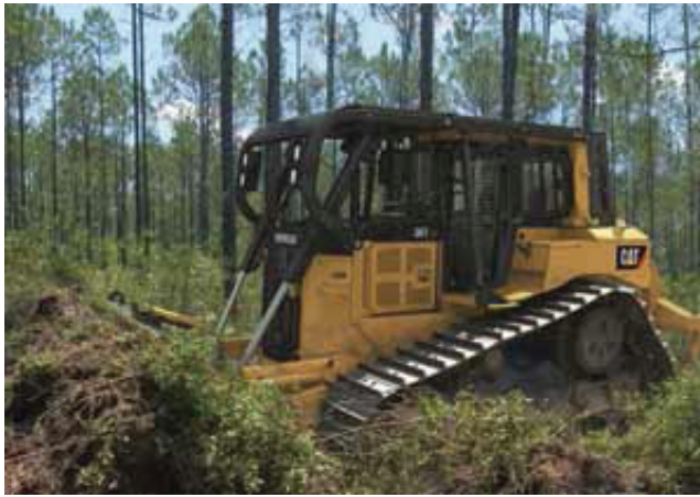
Figure 8-2. Dozer with root rake blade.
