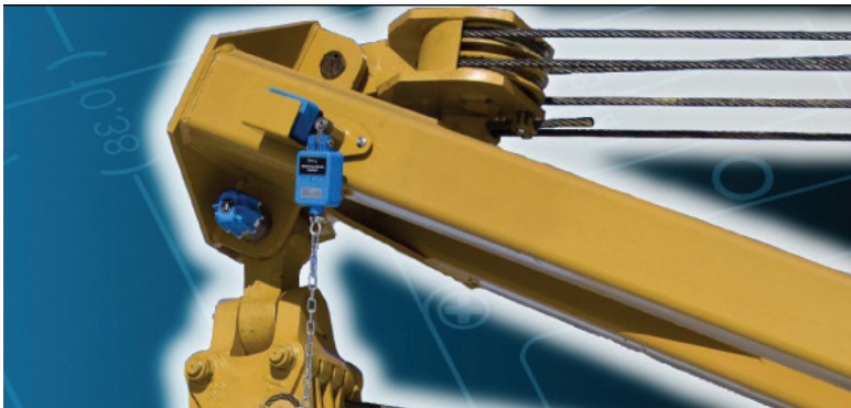
Figure 9-16. Load cell attached to crane provides real-time information regarding the load while it is being hoisted. Source: Cranesmart.
