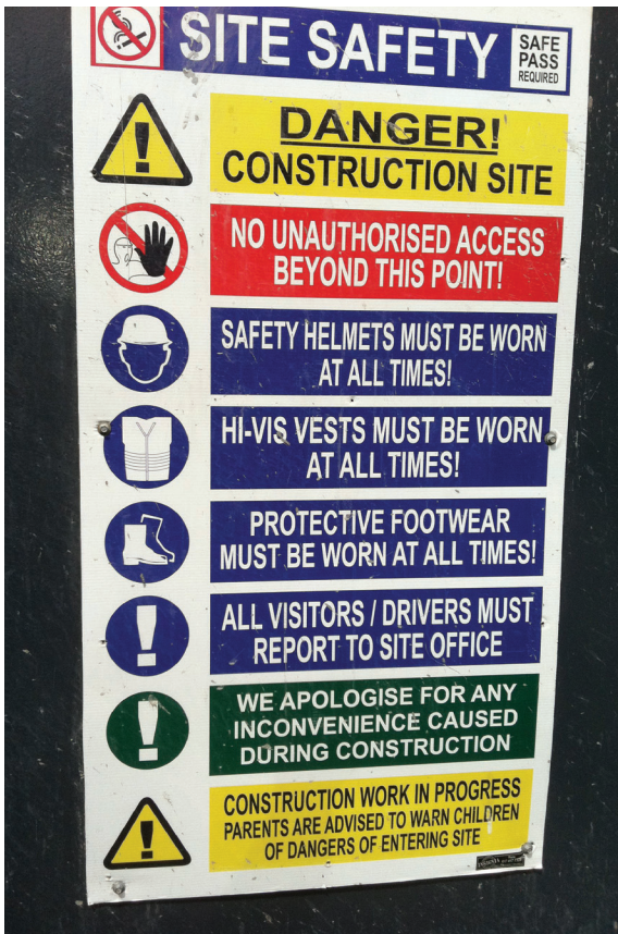
Figure 4-8. Typical site safety signage used during construction.
