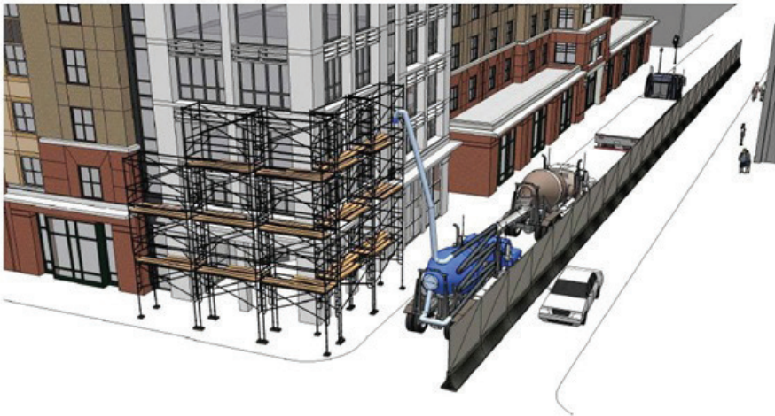
Figure 7-4. Sample BIM to show logistics plan.
