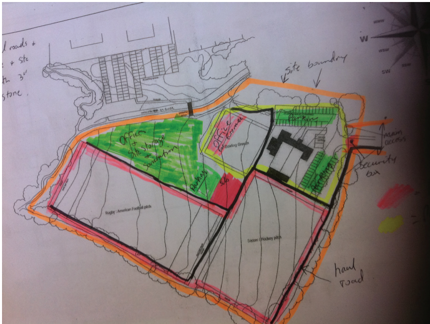
Figure 4-2. Planning the site layout before construction starts.
