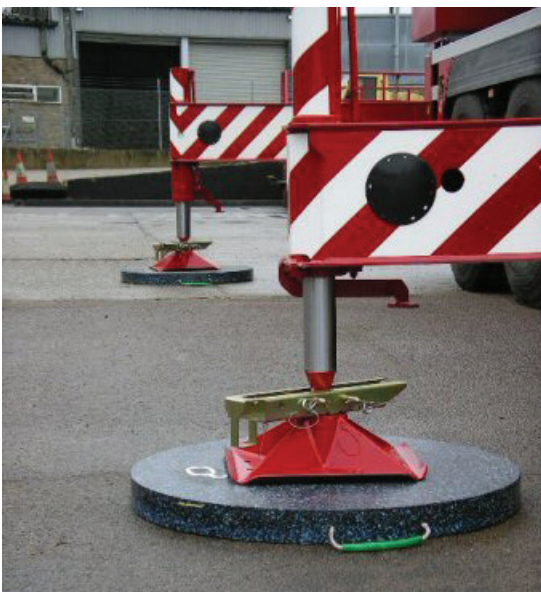
Figure 9-21. Crane supported with dense plastic pad. Source: http://www.outriggerpads.co.uk/specifications.htm .
