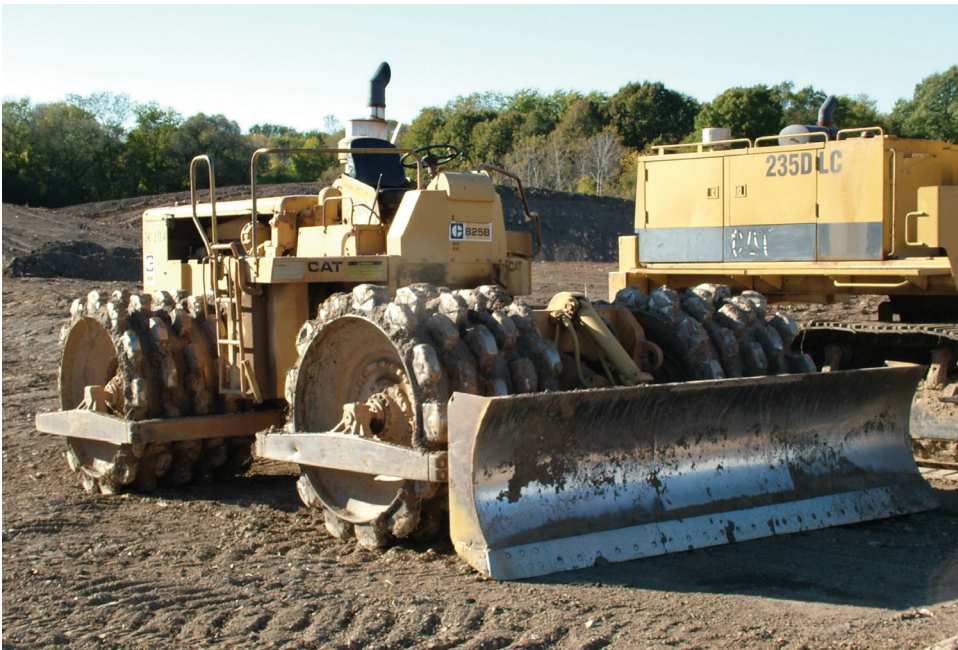
Figure 8-8. Self-propelled sheepfoot roller; no roll-over protective system (ROPS) yet mounted.
