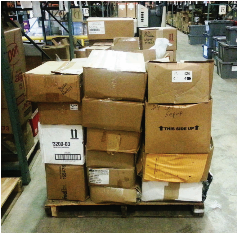
Figure 7-7. Palletized materials not stacked to withstand load or movement.
