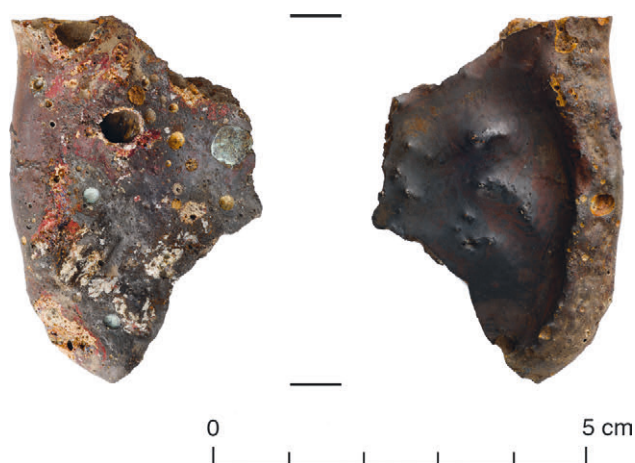
Fig. 7 Plate slags ( Plattenschlacke ) from the smelting site SP 3 at Laas-Platz, with drops of matte on the surface and an all-around elevation with an inner edge at the bottom (photo: G. Gattinger, IUHA, University of Vienna)
