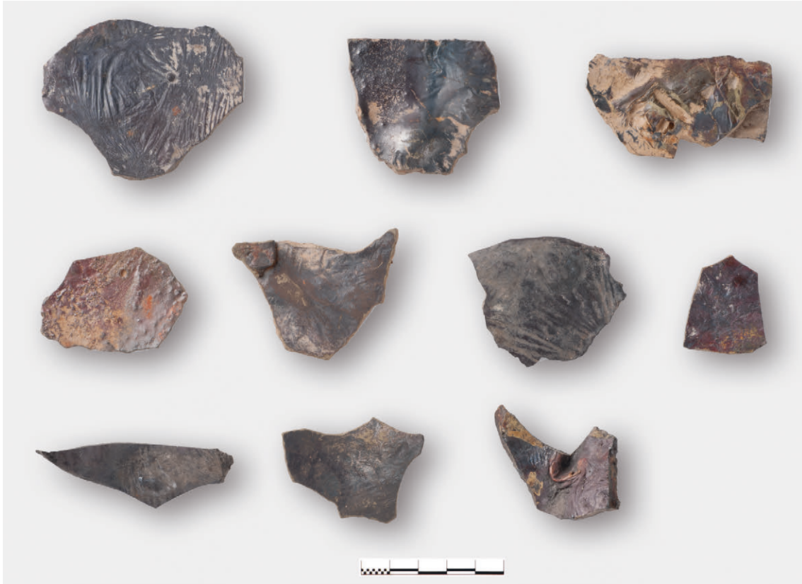
Fig. 5 Plate slags ( Plattenschlacke ) from the smelting site SP 1 at Prader Berg-Vellnair (photo: G. Gattinger, IUHA, University of Vienna; T. Koch Waldner)
