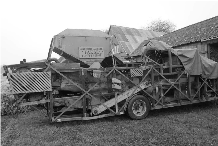
Figure 4.4 Eje has prepared his threshing machine, a Bøje Olsens “langhalmmaskinen Fakse Aps” from Denmark, which he has adapted to fit his needs. In the production of long straw for roof thatching, the grain is a by-product.
