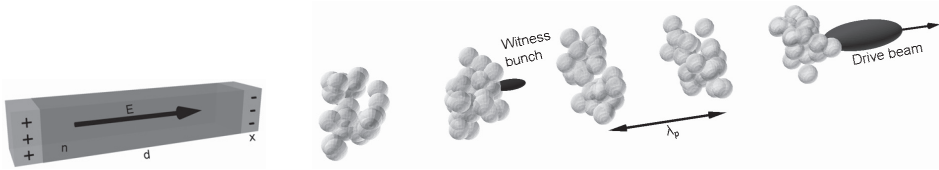
Figure 15.3 Separating charges in a neutral plasma creates an electric field (left). Once excited by a drive beam, the attractive force between the separated charges leads to a wave-like perturbation inside the plasma with very high electric-field strength (right), that can be used to accelerate a witness bunch to high energies.
