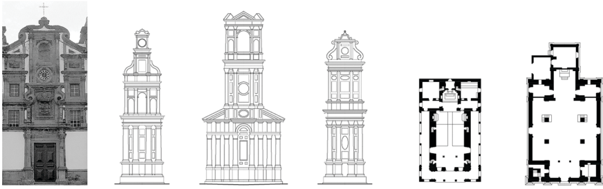
Figure 3.4 (1) Church of St. John, Angra do Heroísmo, Azores. Detail (2) Sebastiano Serlio, Ornamental examples of furniture represented. Book VII (ed. Frankfurt, 1575) (open source). (3) Church of St. John, Angra do Heroísmo, Azores. Plan (adapted drawing) (4) Church of Atouguia da Baleia, Peniche. Plan (adapted drawing).
