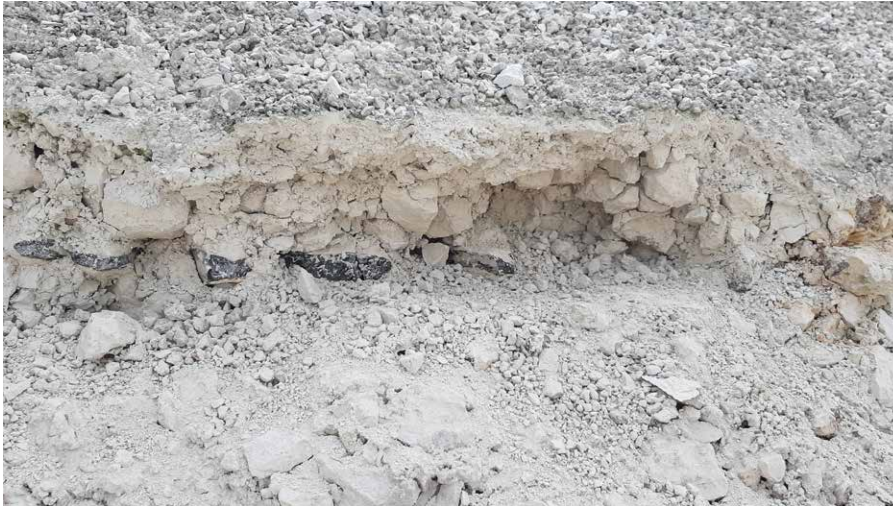
Figure 13. Flint band in a primary deposition at the Hillerslev chalk factory. Recognisable is the fractured state of the raw material due to the strong mechanical forces by the heavy-duty machines (Photo: M. Hinrichs).
