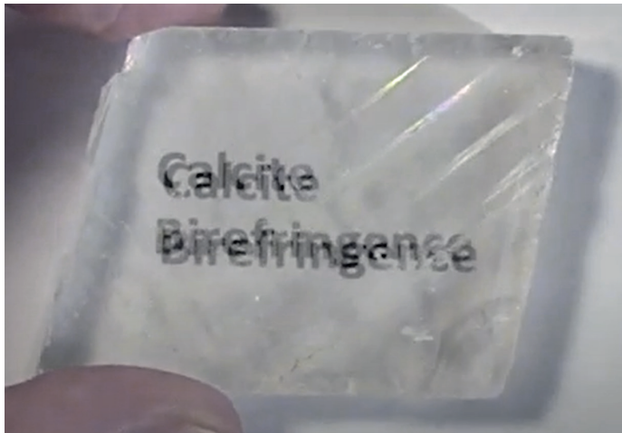
Figure 13.1. Double refraction demonstration in calcite. Source: Photo by author.
