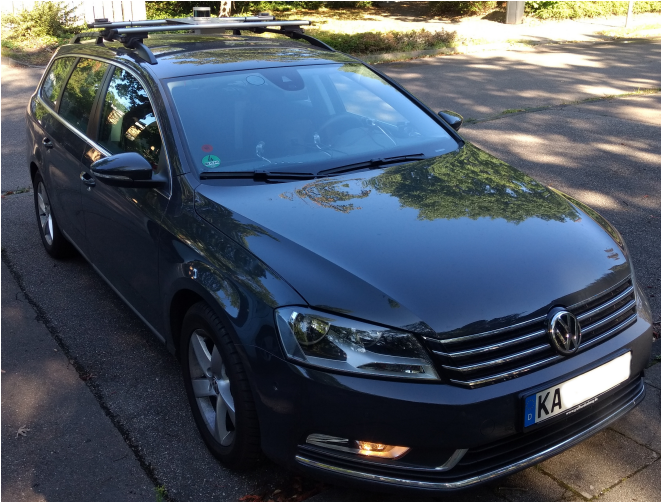
Figure 2.1 Measurement vehicle that was used for the field study. The lidar is mounted on top of the plate on the roof, the IMU is located inside the box below the plate. The two GNSS antennas are placed on the outer ends of the roof railing. The image is a cropped version of the original.
