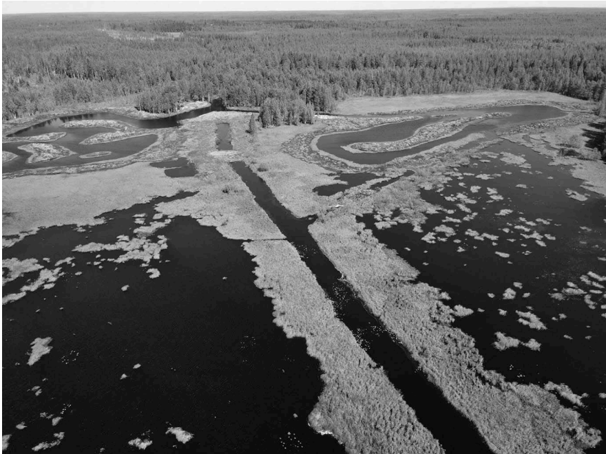
Figure 8.4 Drone photo of Jurvasenlampi Lake in summer 2023. In the middle the historical draining ditch, and in the upper part the new bottom dam, surface-draining peatlands and water-clearing channels are clearly visible.
