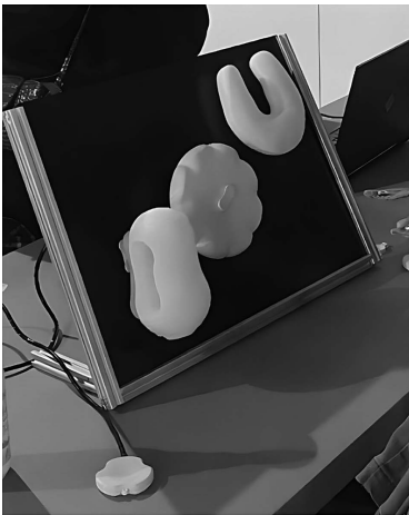
Figure 4.3 The four objects displayed. The portable device for the maintainer, and the three on the workplace (in order: software call, mechanical call, electrical call)
