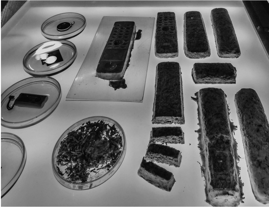
Figure 21.5 This module presents various molds of cell phone cases in which a substrate of hemp and mycelium grows, to fabricate a completely biodegradable product
