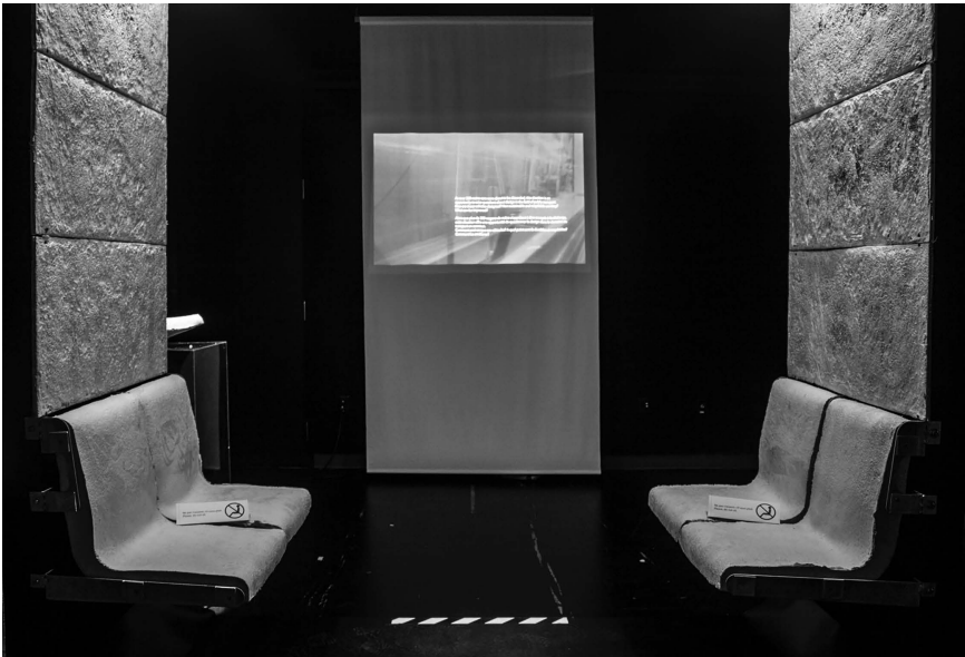
Figure 21.6 Seat and wall panels of a metro car made with a substrate of hemp and mycelium (full-scale model). Research-creation project by Master of Design graduate Théo Chauvirey
