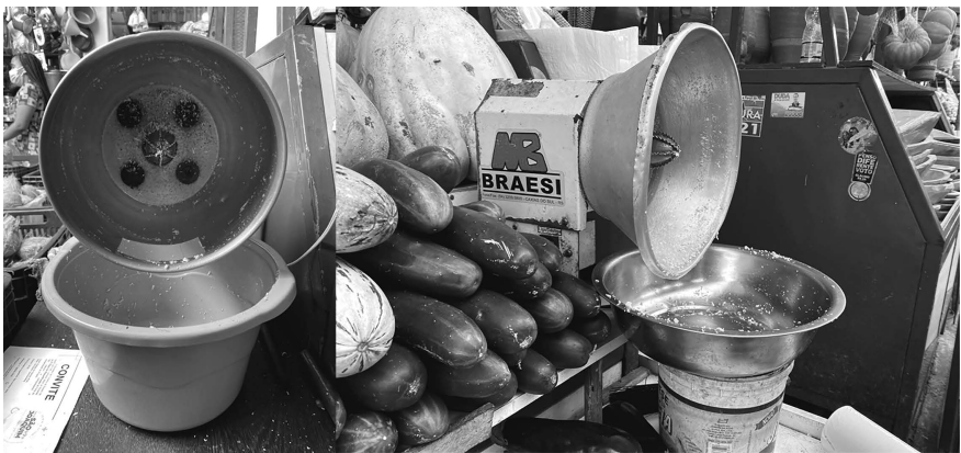
Figure 6.6 Coconut grating machine: product made for grating as assembled from the reuse of a rotational engine and aluminum pan (Photograph: Bruna Dória and Gil Maciel. Nov. 2021)
