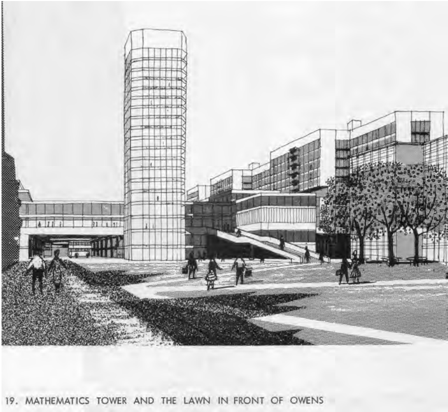
Figure 3.26 Preliminary drawing for the Maths Tower showing the early idea of a ramped access up to an elevated pedestrian realm. Oxford Road is closed on this image and an overbridge connects the Maths Tower to other proposed buildings.
