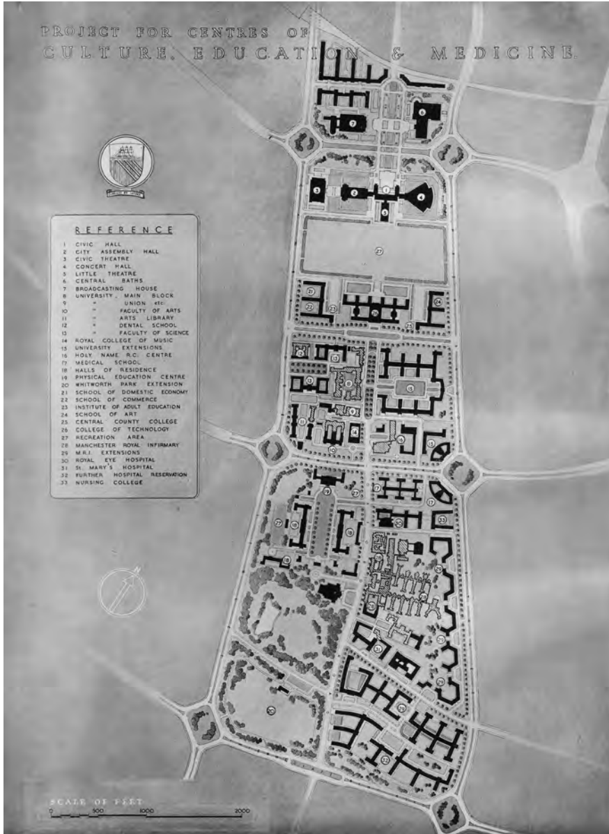
Figure 3.02 Hubert Worthington's plan for the Centre of Education, Culture and Medicine from Manchester's 1945 Plan. The strong axial and symmetrical planning was used to organise the buildings of the 1950s and 1960s along Brunswick Street (labelled '15' on the plan).
