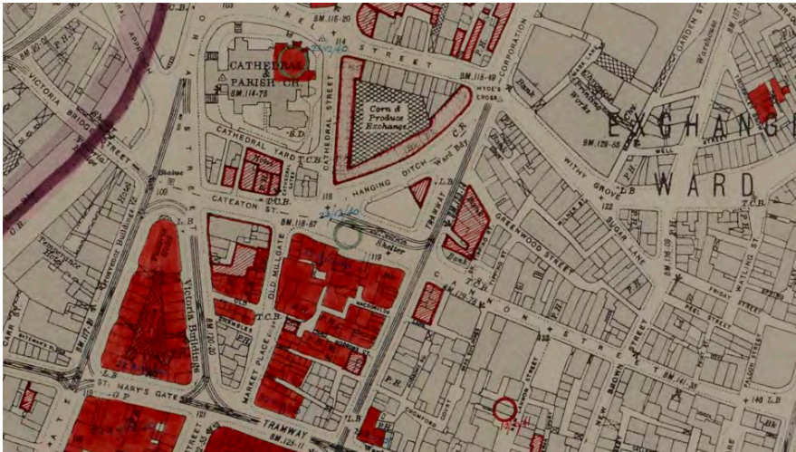
Figure 5.04 Extract from bomb damage maps to show area around Market Place. The buildings shaded in solid red were completely destroyed.
