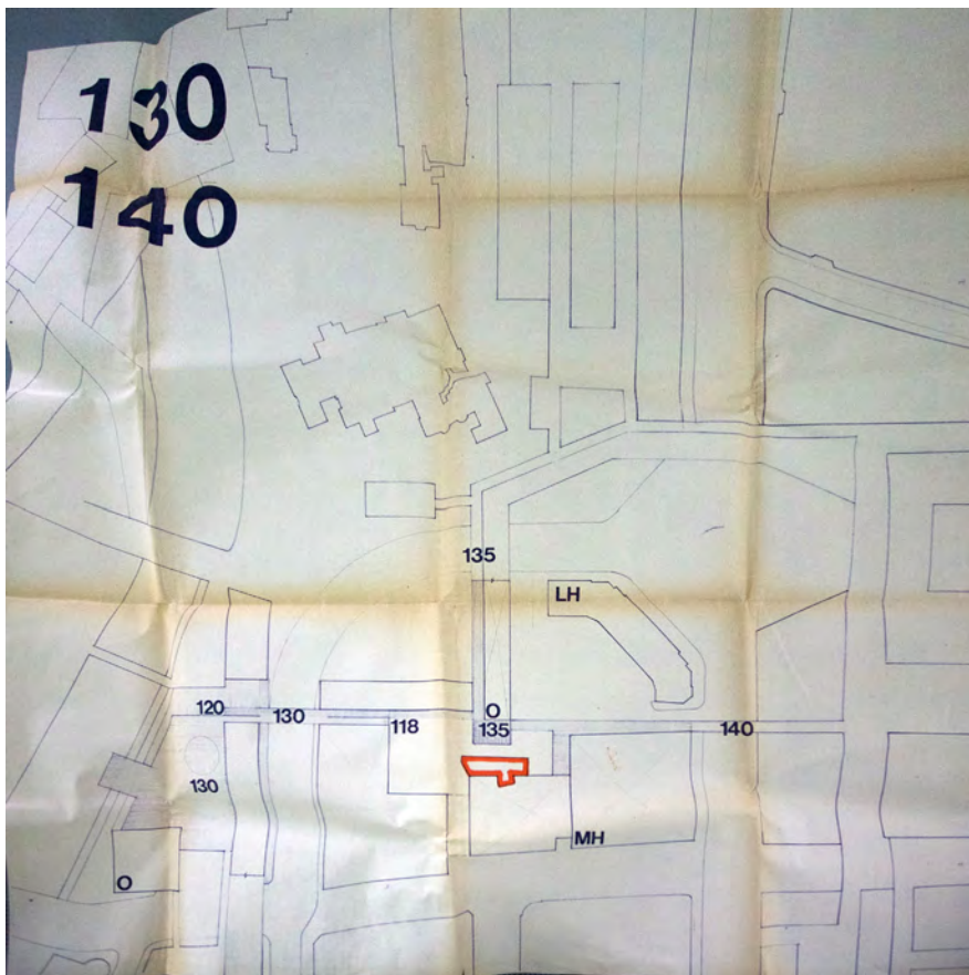
Figure 5.19 Advisory Scheme drawing. The connected nature of the sites to the north, east and west is shown here as high-level bridges at 135m, 140m and 130m above sea level. The apparent title of the drawing is '130 140' and indicates the concerns of the planner and the vertical separation of the city.
