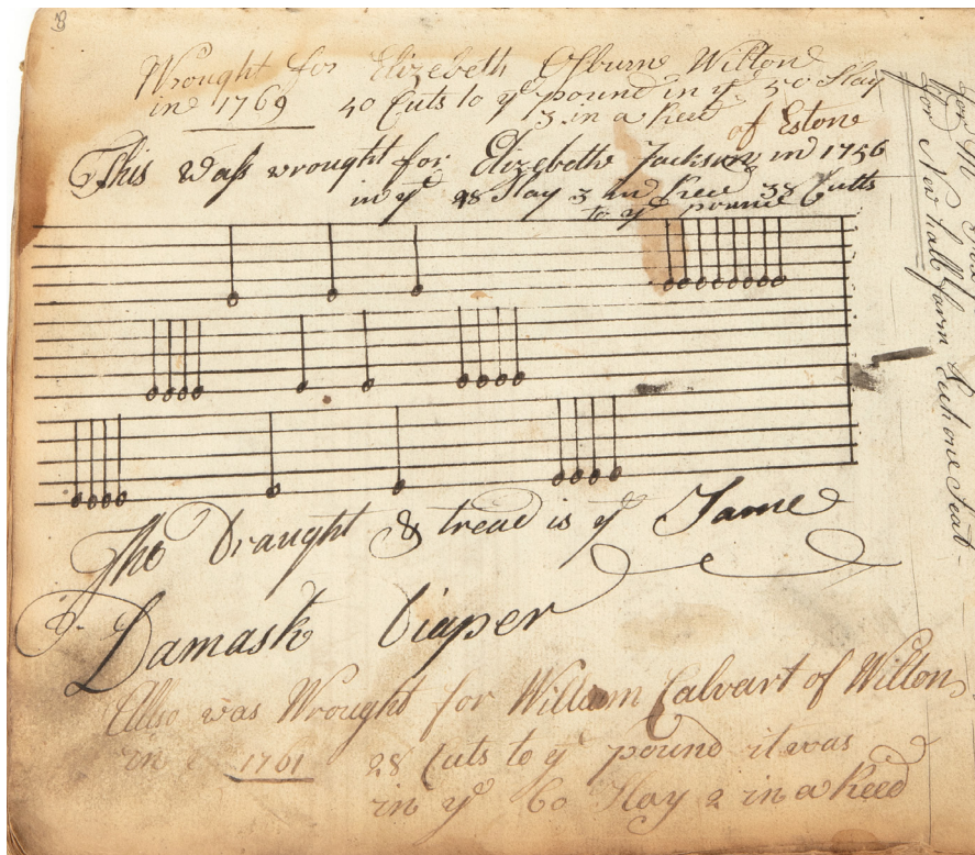
Figure 1.6 Weaver's draft for a linen damask diaper with details of the yarn supplied by customers, from the pattern book of Thomas Jackson, jobbing weaver, Kirkleatham area, Yorkshire, c. 1756. Weaver's thesis book, England, seventeenth–eighteenth century, Cooper Hewitt, National Design Museum, New York, textiles department, 1958–30–1.
