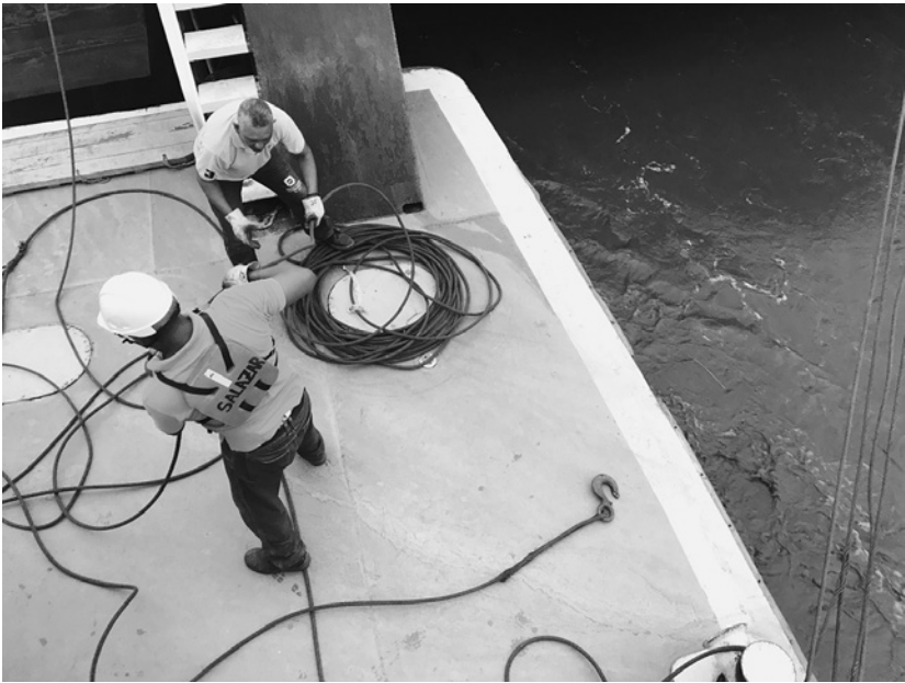
FIGURE 4.6. Marineros (deckhands) maneuvering the cables that bind the barges to the towboat. Source: photograph by author.
