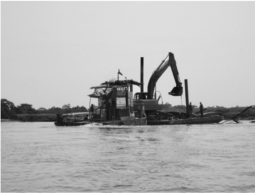
FIGURE 1.4. Dredge rig consisting of a tracked excavator mounted on a pontoon barge. Source: photograph by author.
