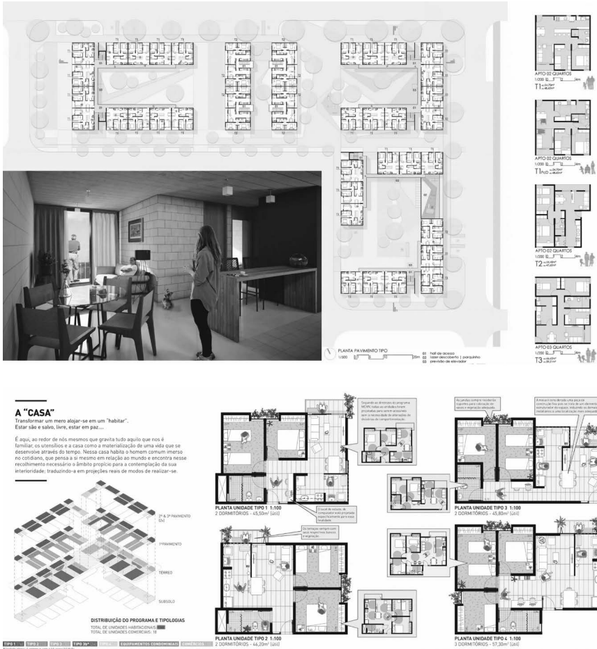
Figure 5.2 Housing typologies. Top: winning project typical building floor and typical apartments. Below: honourable mention project typical apartments.
