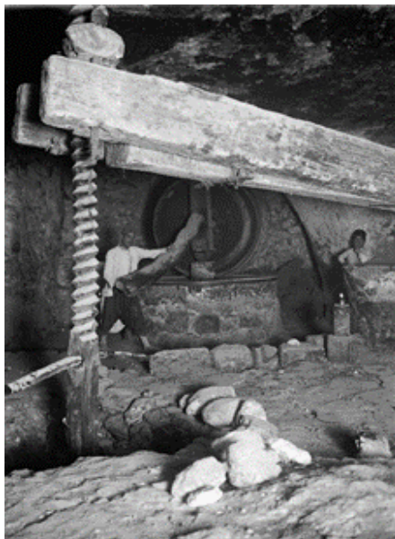
Figure 5: Lever-and-screw olive press operating in Bēt Sāḥūr, 1934–1939 (image: the American Colony, Jerusalem, G. Eric and Edith Matson Photograph Collection, accessed 26 December 2024, https://www.loc.gov/pictures/item/2019694385 )
