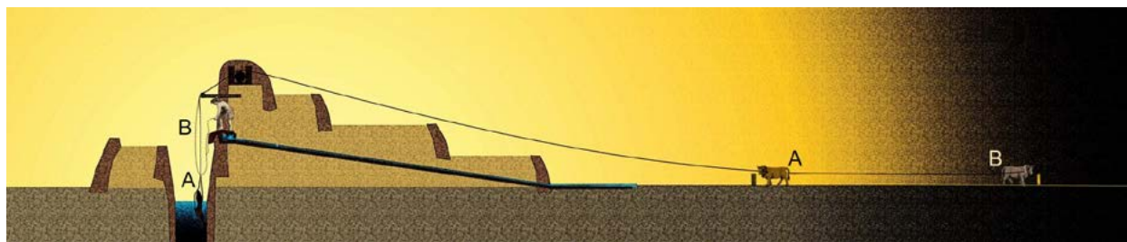
Fig. 6 – Graphic illustration of withdrawal and elevation of water (magrod) used in Ifni (Morocco). At position A, the draught animal is near the well and the goatskin bag is lowered into the water. At position B the animal pulls the bag to withdraw the water. The well at the motilla of Azuer might have been of this kind and would have been exploited in the same way. – (Drawing: Authors’ design).
