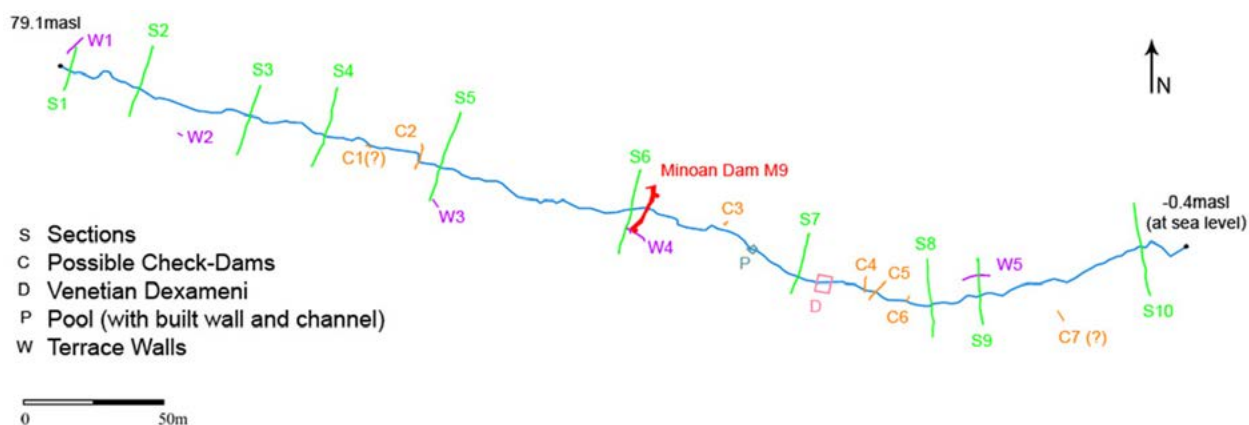
Fig. 12 – Water-management system in Dune Creek Ravine, including Dam M9 at the centre and several check-dams. – (after Betancourt 2012: 26, fig. 13).
