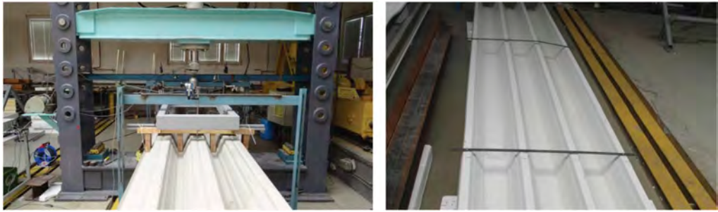
Figure 4. View of the test stand and transverse ties (stabilizing the sheet).
