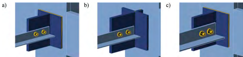
Figure 2. Boundary conditions of steel angles: a) A1–A3: rigid, b) A4–A6: uniaxially hinged, c) E1–E3: rigid.
