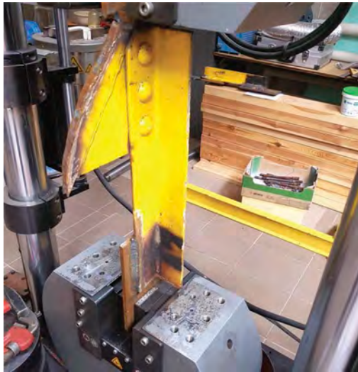
Figure 3. Element during bearing capacity tests of the riveted joint.
