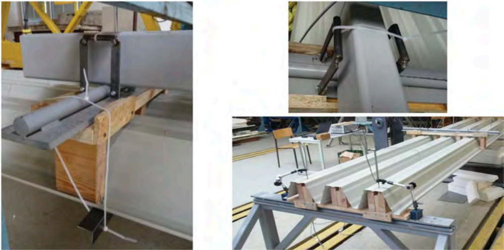
Figure 3. The supporting elements.
