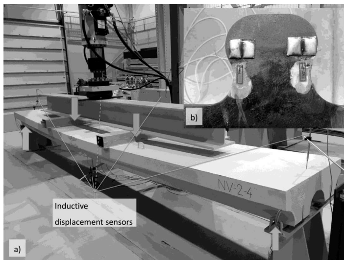
Figure 5. Four-point flexural test: a) the overall layout of the test; b) strain gauges application on the tooth of the strip.
