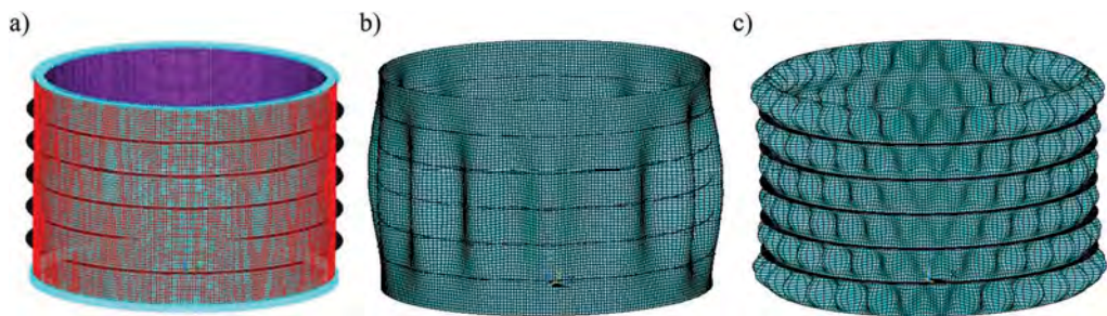
Figure 1. Types of instability or failure in ring-stiffened cylindrical shells subjected to external pressure. a) Ring-stiffened shell under uniform external pressure, b) Overall buckling of the whole shell system, c) Local buckling in the shell wall between stiffeners.
