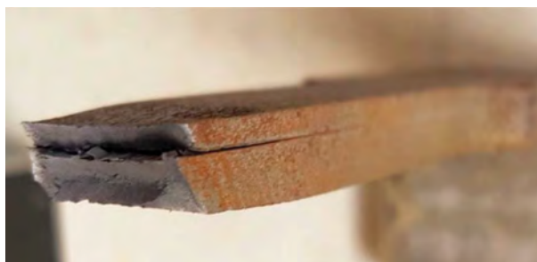
Figure 4. Steel sample that underwent lamellar tearing as a result of strength tests.
