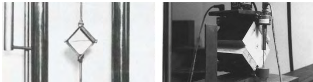
Figure 1. Square tests by Jungbluth & Berner (1986, Bild 7.21) and Davies (2001, Fig. 13.4).
