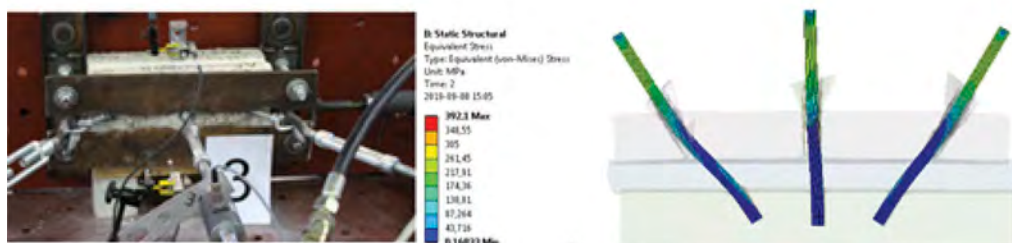
Figure 6. Failure models of three-anchor anchorages bonded at an angle of 60 degrees: experimental test and FEM model.
