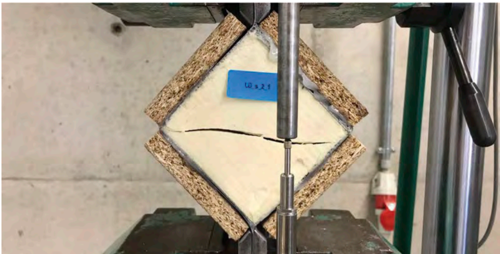
Figure 4. Plastic hinge square shear test – Shear fracture.
