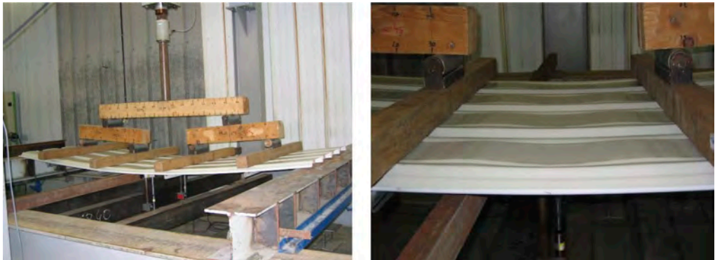
Figure 13. Example of testing of trapezoidal sheeting under bending moment.
