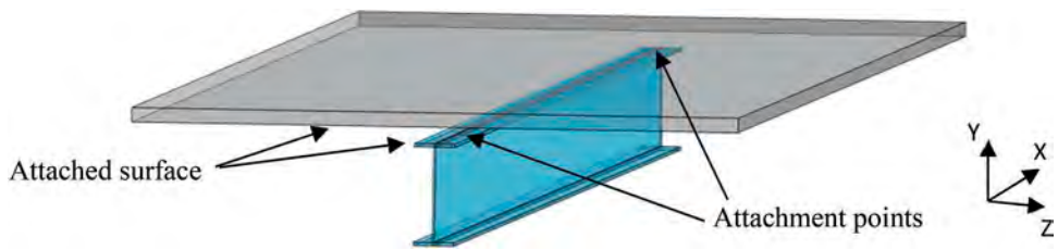
Figure 2. Attachment points of the FE model corresponding to the location of the shear connectors.
