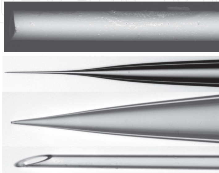
Fig. 2. Electron and optical microscopy images of pre-processed (top) and conventionally processed capillaries.
