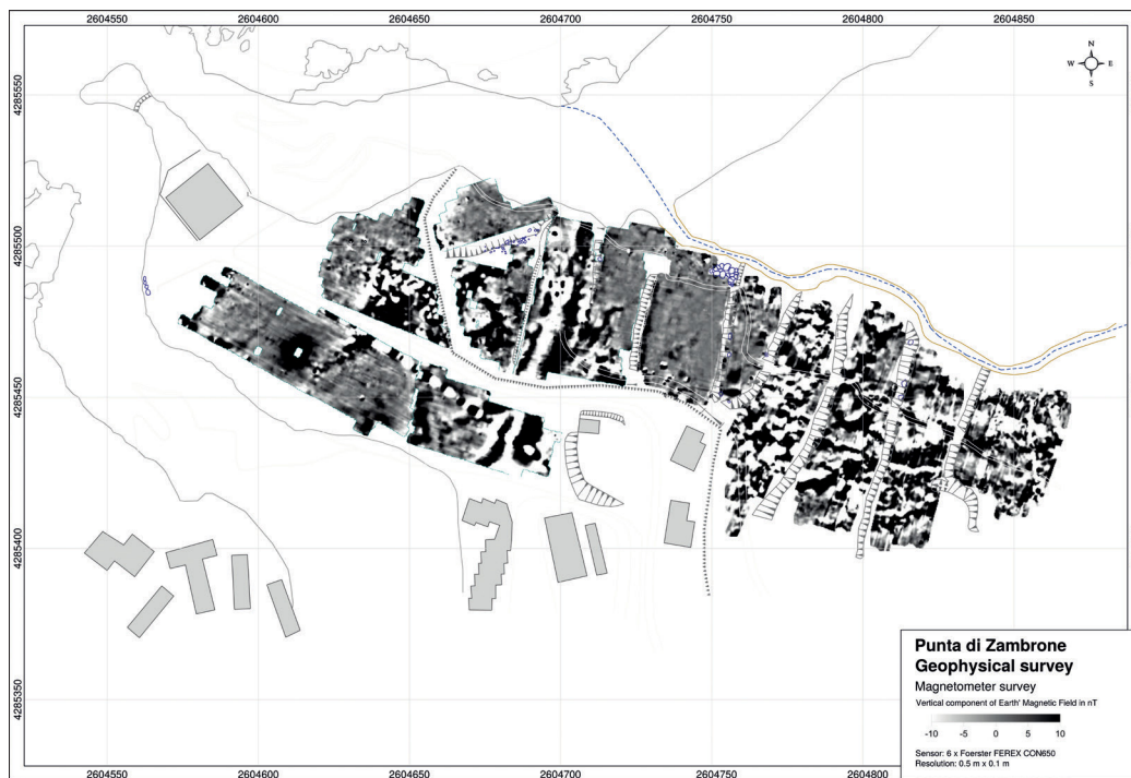
Fig. 5 Data of the magnetometer survey in a \pm 10\text{nT} dynamic (graphics: B. Ullrich)
