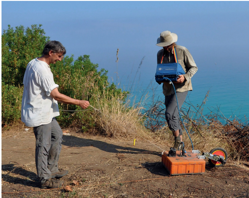
Fig. 3 GPR survey on Terrace E using the SIR-3000 and a 270-MHz antenna (photo: R. Jung)
