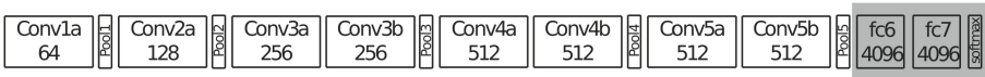
Fig. 1. C3D model, taken from Tran et al. [30]. Convolutional layers, denoted Conv , feature kernels of size 3 \times 3 \times 3 and stride 1 for all dimensions, respective filter sizes are shown in the image. Max-pooling layers, denoted Pool , feature kernels of size 2 \times 2 \times 2 , except for Pool1 with a kernel size of 1 \times 2 \times 2 . Fully connected layers fc , highlighted in gray, were removed from the network and weights of the convolutional layers were kept fix.
