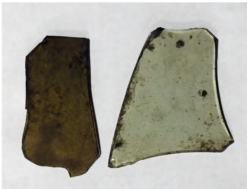
7 Two types of glass found at Aden, a late 16th-century Presbyterian meeting house in Aberdeenshire. The dark green sample is HLLA1 and the clear piece is a sample of HLLA2.
