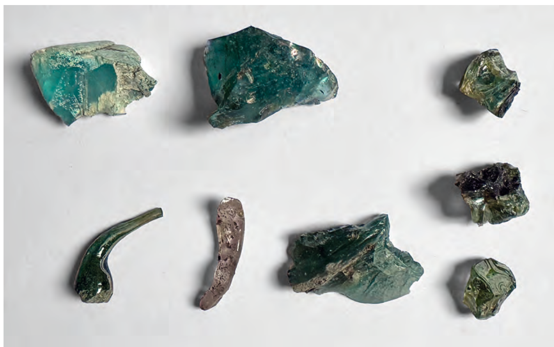
4 Pieces of glass waste excavated from the 1690s glass furnace at Morison's Haven.
