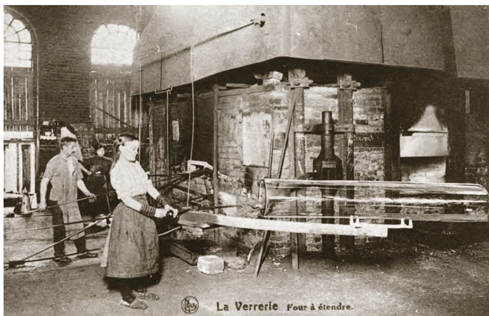
7 Placing glass cylinders into the annealing kiln, late 19th or early 20th century, Belgium, photographer unknown.
