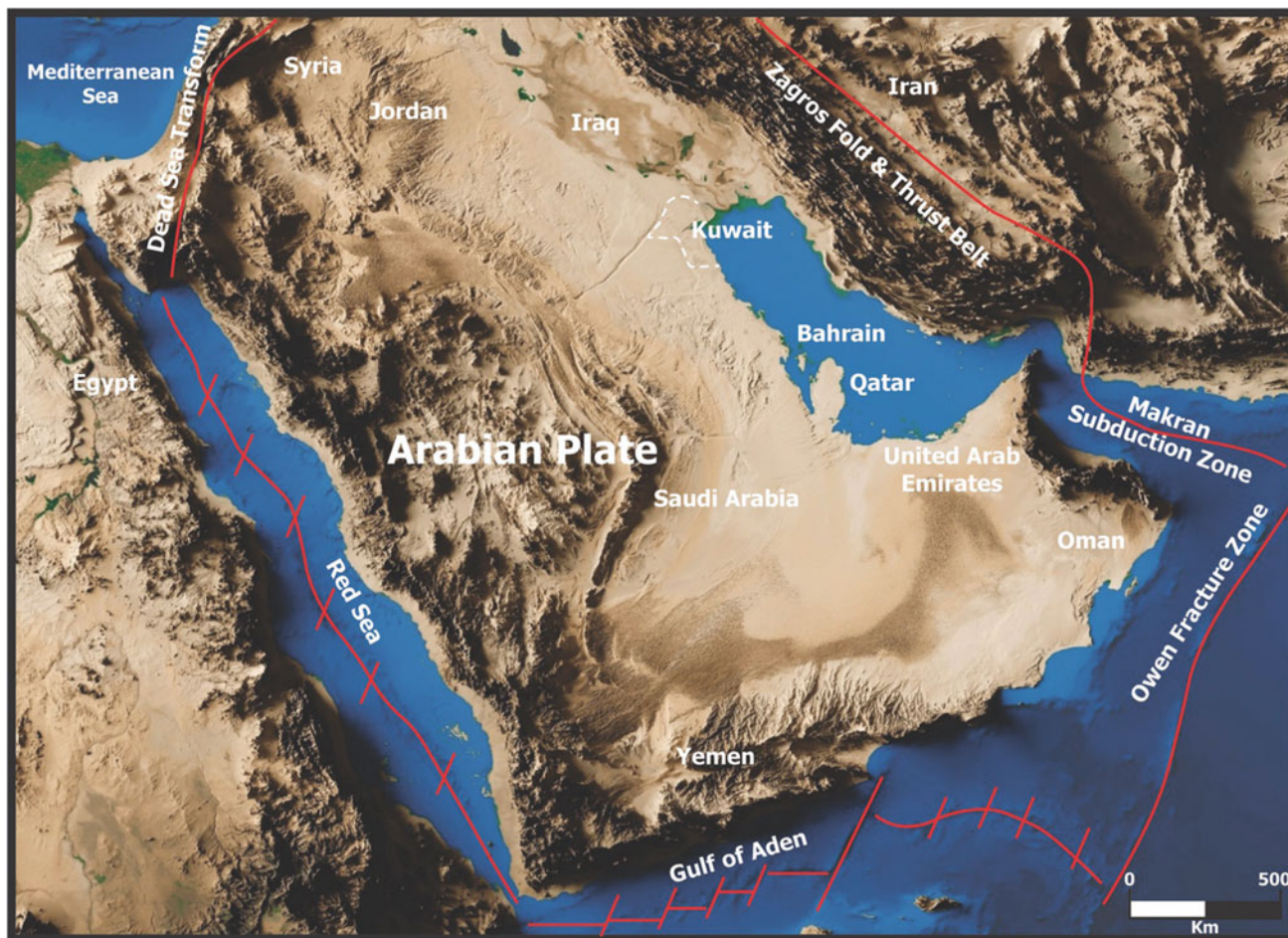
Fig. 5.1 Digital Elevation map of the Arabian Plate with the main plate boundaries. The Arabian Plate is bounded from the northeast by collision margin of Zagros Fold and Thrust Belt. Rift margin to the west
