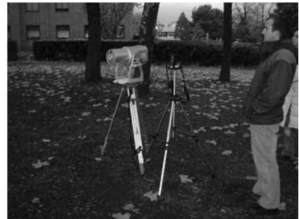
Figure 3. The Laser scanner and the camera at the same height
