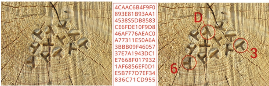
Fig. 9.7 The coded brands punched in the solid wood on the left carry an information carried as a unique ID for the log as simplified on the center and right. (Source www.otmetka.com )
