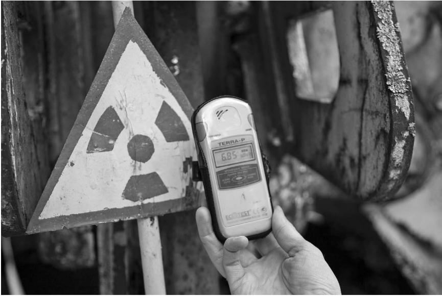
Figure 4.10 Measuring radiation at a hotspot.
