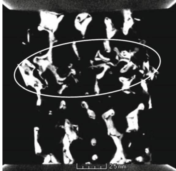
Fig. 16.13 Reconstructed cross section after 20% compression [11]
