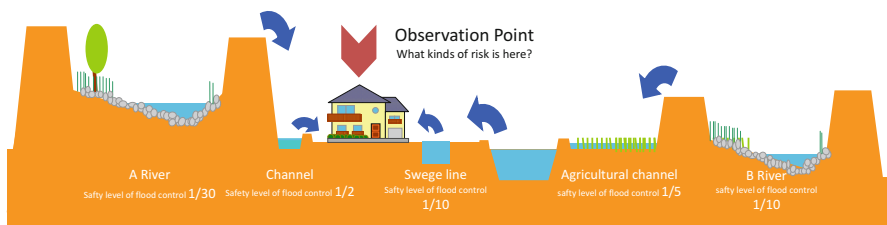
Fig 4.4 Site safety level. This is the level of safety of a point surrounded by a river/channel complex and for the setting of daily life (Source: Taki et al. 2010)
