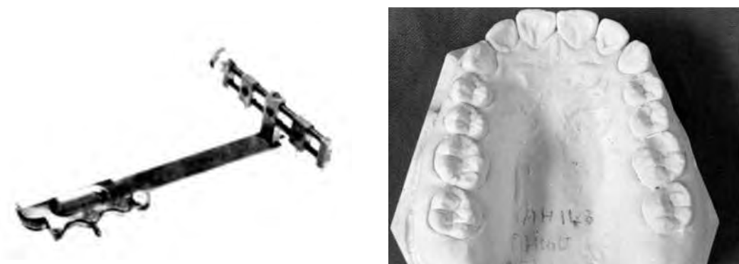
Figure 4.7 Instrument used for measuring arch breadth and depth on dental models during the 1960s
