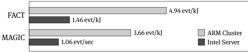
Fig. 5.9: CORSIKA energy efficiency observed when processing FACT/MAGIC events on 160 ARM cores (“ Eriador ”) vs. 48 Intel Xeon cores.
