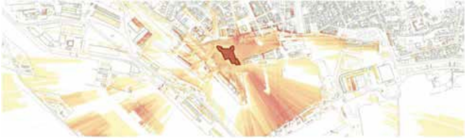
Figure 5 - Example of visual influence of the old fortress of Livorno performed in the GIS environment with the View Sheed Analysis.
