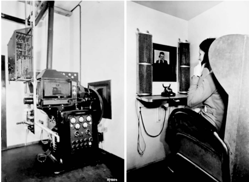
Figure 4 a–b: Camera setup behind the booth (left) and booth of the German Fernsehsprechdienst in the late 1930s (right)
