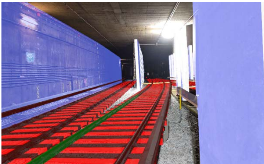
Figure 8: Screenshot of the 3D BIM model, as visualized on-site with DigiTAR
