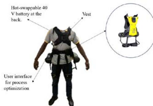
Fig. 2: Active (CrayX) back-support exoskeleton.
