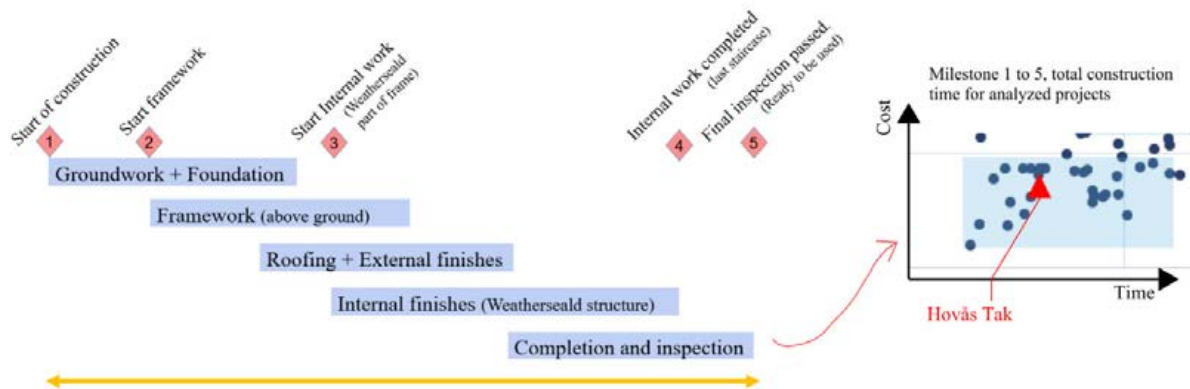
Fig. 3: When having the same WBS and coding, it is possible to analyze projects KPI's against each other to find outliers.
