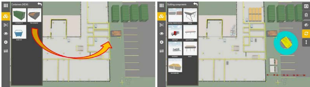
Fig. 5: Adding prefabs using drag-and-drop (left), and context menu and rotation gizmo (right)
