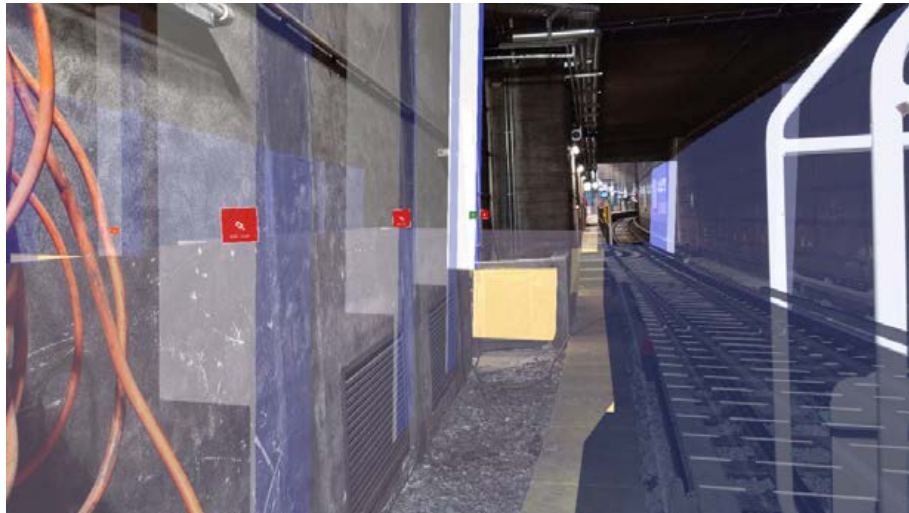
Figure 9: Screenshot of QC tags visualized on-site with DigiTAR
