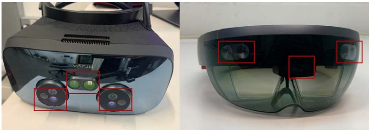
Figure 1 Inside-out systems rely on a group of cameras and/or sensors manufactured into the headsets. These systems do not depend on any external sensory information.
