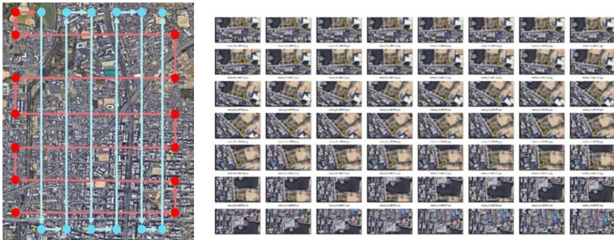
Fig. 8: Waypoints specified by our KML file depicted on Google Maps (Osaka: Suita, Japan) (left) and the captured virtual aerial photos through the waypoints in Google Earth (right)
