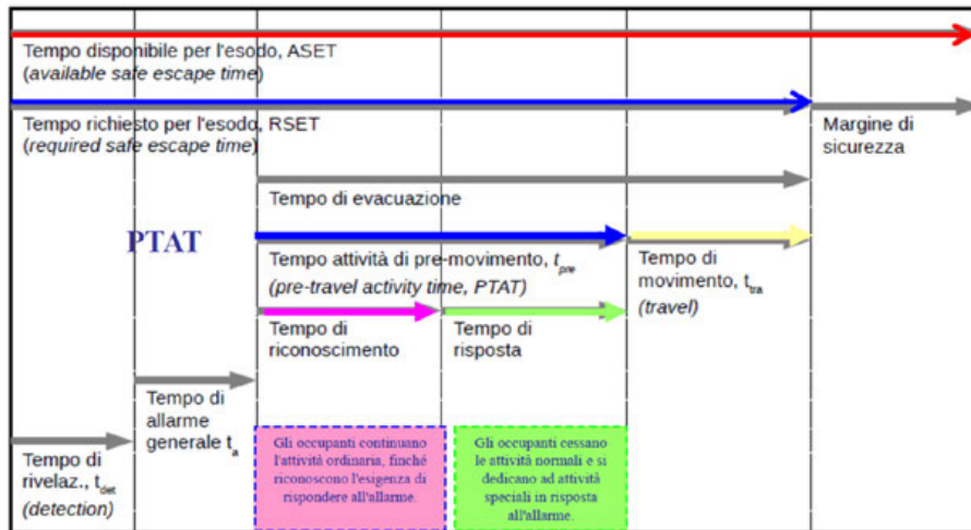
Fig.5 - Comparison between ASET and RSET (Illustration M.3-1 of the Code DM 2019, October 18, modified)
