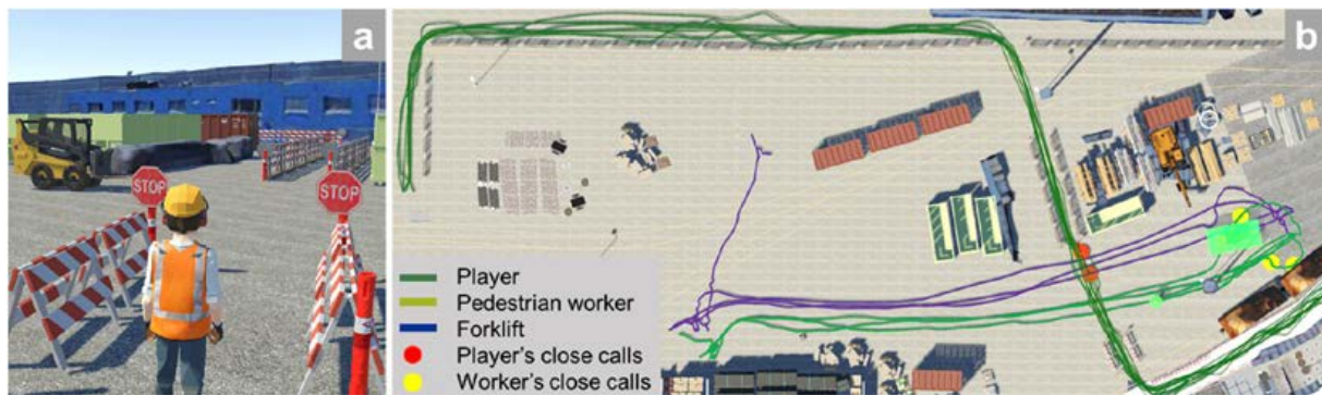
Fig. 6: (a) Results of the first training scene, including the landscape, BIM model, resources, and trajectories from IoT devices, and (b) the trainee crossing the road while the forklift follows the real-world trajectory.
