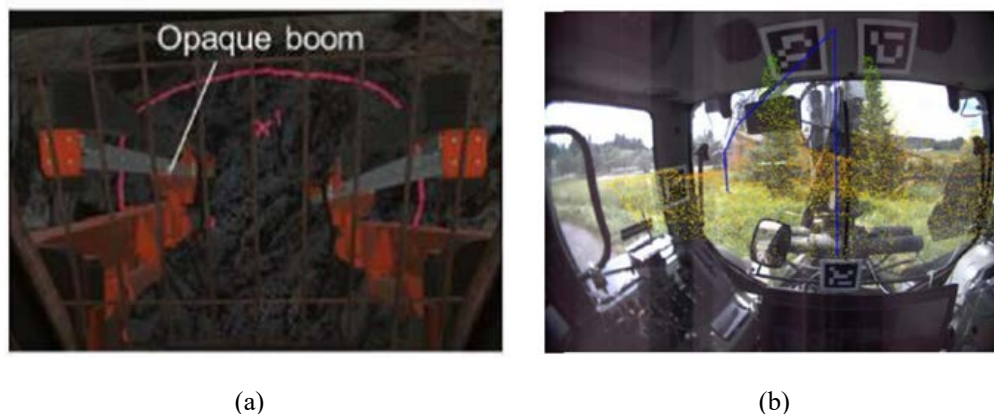
Fig. 1. (a) See-through visualization of the boom presented in (Aromaa et al., 2020) , (b) Visualization of the environment using point cloud presented in (Palonen et al., 2017)
