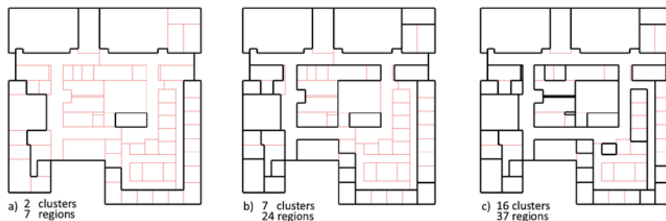
Fig. 7: Different thermal zoning schemes based on different cluster distance.
