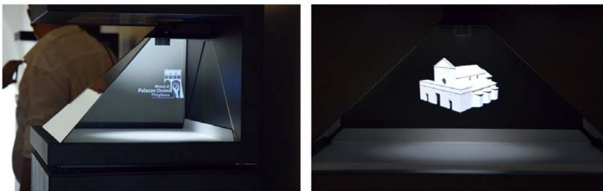
Fig. 15: The showcase shows the holographic projection of the video, as indicated by the sequence of frames.
