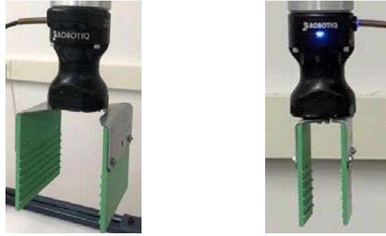
Figure 3. The prototyped robotic end-effector at Fully open position (left) and at fully closed position (right).
