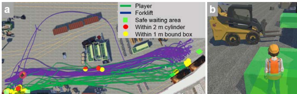
Fig. 7: The (a) results from Training Scenario 2 indicating the trajectories and proximity events, and (b) safe waiting areas where the trainee can safely wait for the return of the forklift until its standstill.
