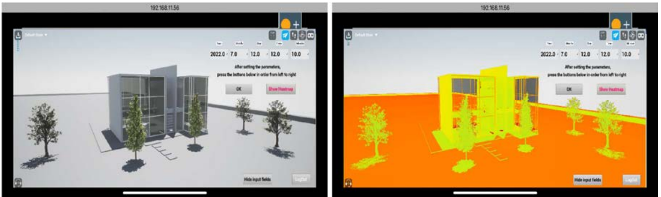
Fig. 3: CG of ground shading with standard diffuse reflection (left) and resultant WBGT heat map (right)
